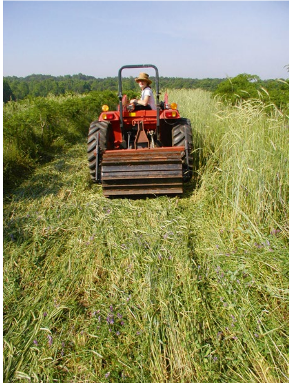
Fig. 4.7 A roller crimper being towed behind a tractor. The angle irons crimp and kill the rye, preventing it from sprouting
