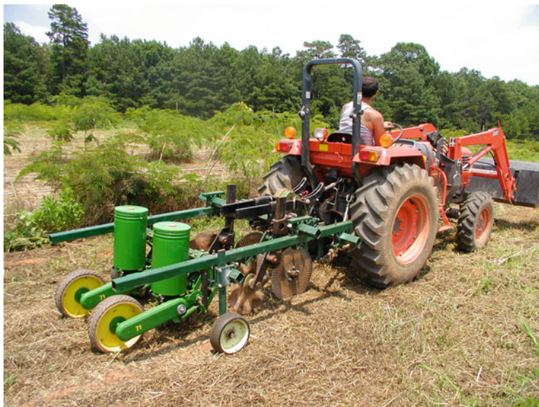
Fig. 5.1 A no-till planter used to plant corn or beans directly through the residue of a winter cover crop, in this case, crimson clover. For strip tilling, the shanks can be lowered to open narrow strips of mineral soil. The seeds are inside the hoppers and drop out into a slit opened up by the coulter wheels preceding the hoppers. Tamping wheels behind the hoppers close up the slit. In South Georgia, no-till planters can consist of 16 or more hoppers on the same piece of equipment
