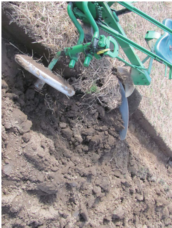
Fig. 2.2 Close-up of a moldboard plow, moving right to left. Note the curved steel blade of the plow which actually inverts the soil. Turning over the topsoil makes it a good seed bed, and buries the weeds
