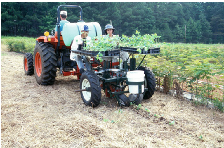
Fig. 5.2 A no-till seedling transplanter. The two workers take seedlings from the pots on the tray and place them in open-top, clamp-like spades hanging from a ferris-wheel- like device between them. As the wheel rotates and a spade enters the soil, the spade opens up and the seedling drops out. The tamping wheels close the soil. The tank of water behind the tractor supplies a shot of water as the machine moves forward
