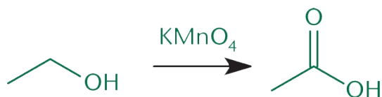
Figure 8.8. Synthesis of a Carboxylic Acid via Oxidation of a Primary Alcohol
