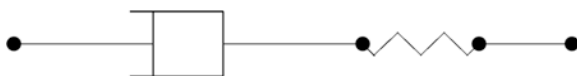
Fig. 8.5 The Maxwell model for visco-elastic media consists of a viscous damper (on the left ) in series with an elastic spring (on the right )
