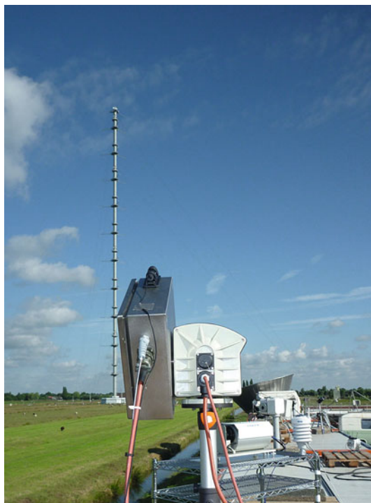
Fig. 7.12 One of the more than 20 MAXDOAS-like instruments in use during the Cabauw Intercomparison campaign of nitrogen dioxide measuring instruments (CINDI), June–July 2009, Cabauw, The Netherlands.
