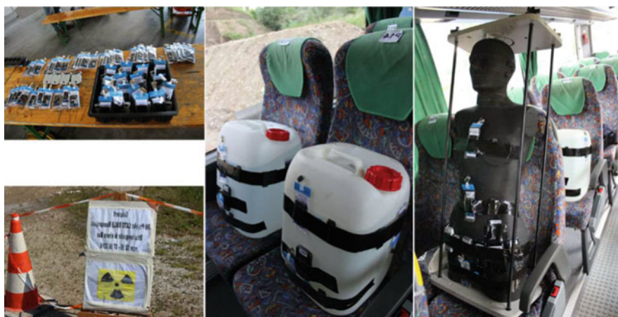
Fig. 2 Thermoluminescent dosimeters (TLDs) and electronic personal dosimeters (EPDs) (upper left corner), water canisters equipped with TLDs and EPDs (center), and an anthropogammametric phantom used to assess the organ doses (right)
