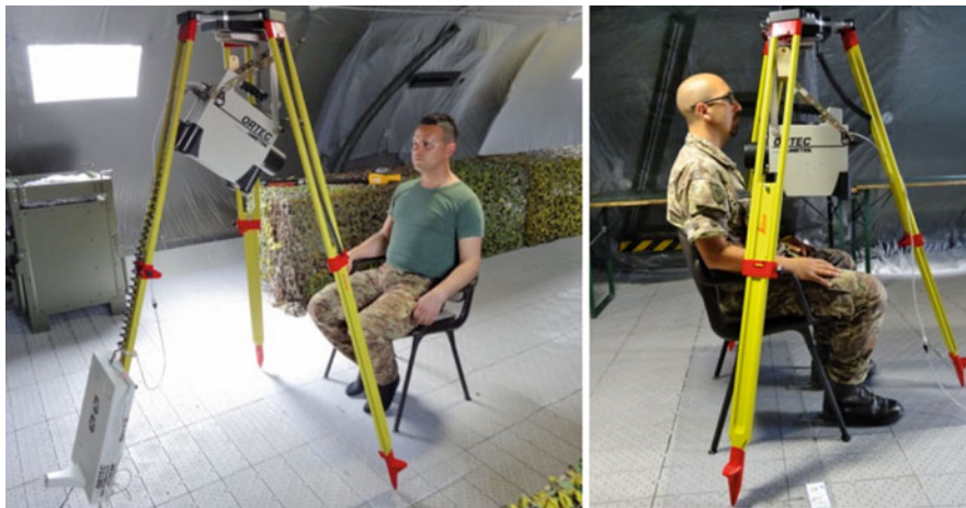
Fig. 4 Trans-SPEC-DX-100 spectrometer in sitting WB (left) and T (right) configurations
