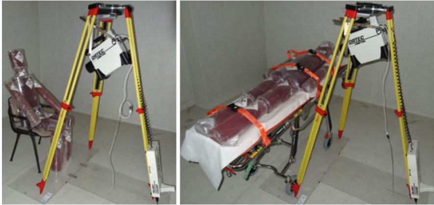
Fig. 2 Geometry calibration in sitting WB (left) and in supine WB (right) configurations
