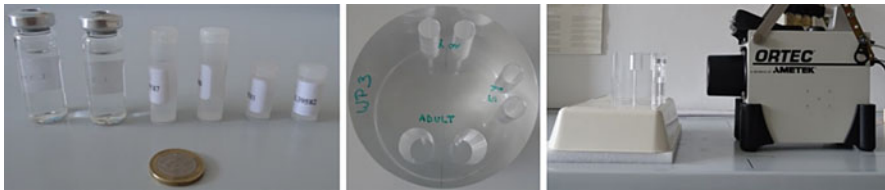
Fig. 3 Three pairs of vials in liquid form simulating different thyroid sizes (left) to be inserted in the neck plexiglass phantom (center) for calibration in T configuration (right)
