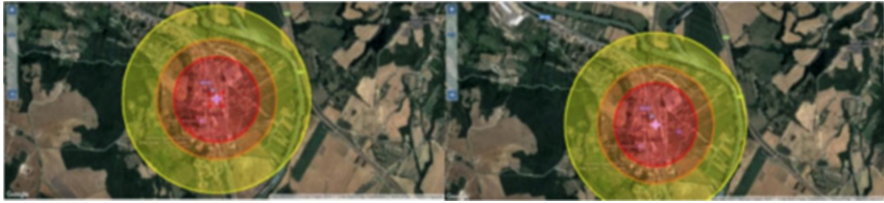
Fig. 2 BLEVE generated by butane and propane
