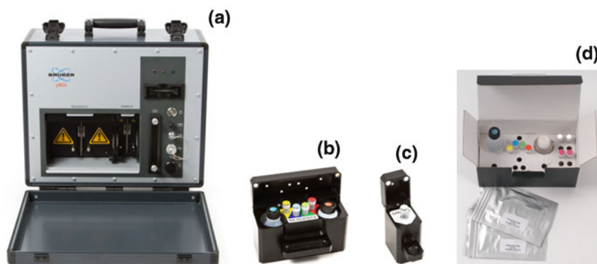
Fig. 1 The pBDi open (a) with reagents (b) and a sample holder (c) as well as a training kit (d)
