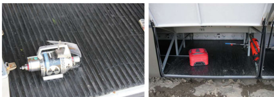
Fig. 3 One of the configurations tested consisted of an unshielded source inside a suitcase and deployed in the cargo bay of the bus
