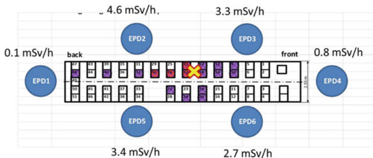
Fig. 4 These are the EPD dose rates measured outside the bus. The driver seats are on the right-hand side of the figure, and the engine block is on the left. The yellow X marks the place where the source was located
