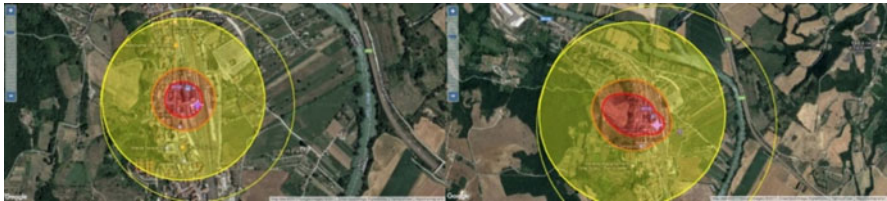
Fig. 4 Shock wave generated by detonation (left butane, right propane), different colors with different intensity, from the highest (red) to the lowest (yellow)
