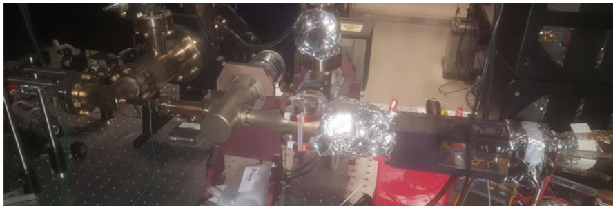
Fig. 2.6 The old vacuum chamber in the first generation KRb experiment. The vapor cell MOT area is on the right, and separated by a large differential pumping section and a gate valve is the science cell side
