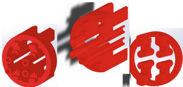
Fig. 7.3 The front macor holder in the science cell. The hole diameter for the rods is 1 mm, and the entire diameter is \approx 15 mm. The groove on the front side holds the ITO-coated plates
