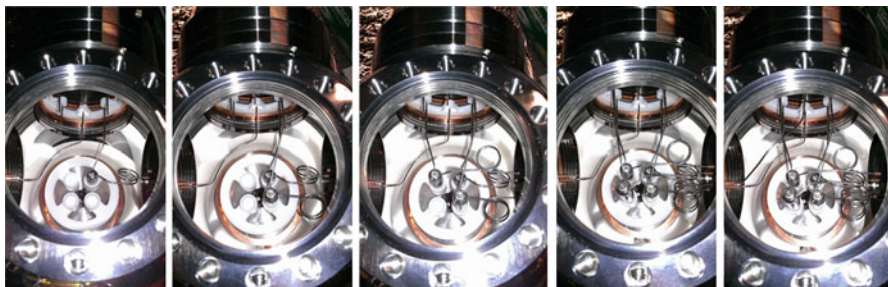
Fig. 8.19 Assembly of the capacitors and inductors and their connection to each other and the transmission line to the science cell. These images show a time sequence left to right of each successive electrode being connected
