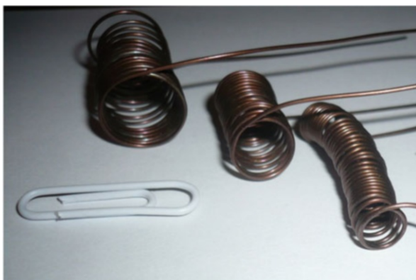
Fig. 18.6 Metal columns can be coiled in small diameters, allowing very small oven configurations
