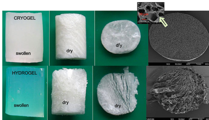
Fig. 5 Images of the cryogel ( top row ) and hydrogel samples ( bottom row ) formed at -18 and 50 °C, respectively, in swollen and dry states. C_{SF} = 4.2 wt% EGDE = 20 mmol/g; TEMED = 0.10 %. Scale bars: 1 mm (SEM images on far right ), 20 \mu\text{m} ( inset ). (From [50] with permission from the American Chemical Society)
