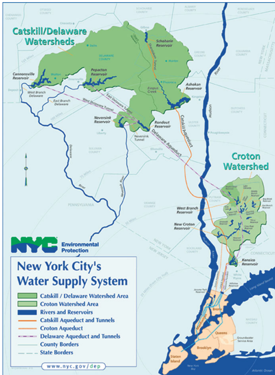
Fig. 2 New York City's water supply system. Water to the city of New York is gravity-fed, predominantly from the Catskills. Because of this use of gravity and the high initial quality of the water, New York City has a highly energy efficient water supply system. Used with permission of the City of New York and the NYC Department of Environmental Quality
