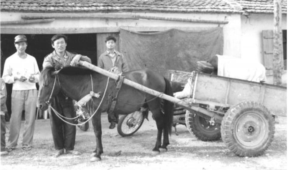
Figure 1. Cart harness in Viet Nam (note 'breastband', cart loaded behind centre of gravity and lack of breeching straps for braking).
