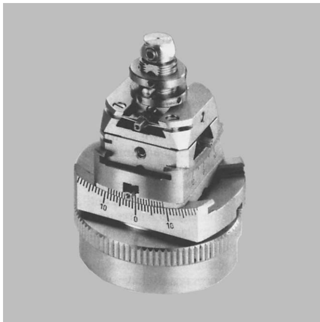
Figure 1.11. A goniometer head.
