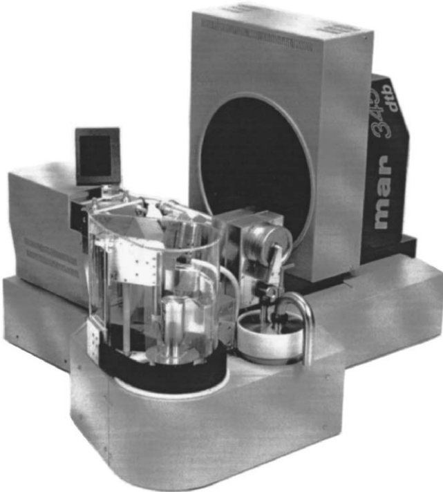
Figure 2.10. (a) The principle of the image plate as an X-ray detector. (b) The image plate instrument produced by Mar Research. It has a circular plate behind the black area where the plate is protected from daylight. For scanning, the plate rotates and the laser scans it along a radial line. In front is the cryogenic sample changer. (Courtesy of Mar Research, info@marresearch.com )
