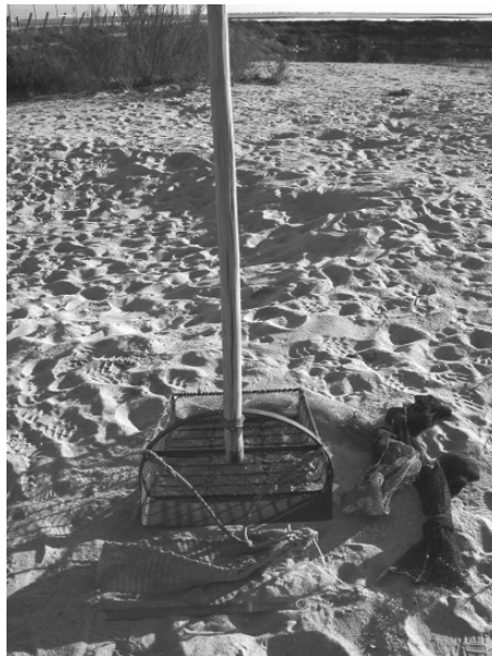
Fig. 5.1. Photograph of the manual dredge used in the Donax trunculus fishery along the Portuguese south coast
