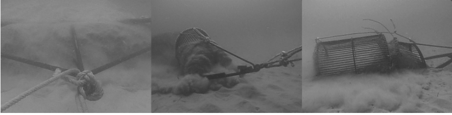
Fig. 5.11. Underwater photographs of the north dredge (left), net-grid traditional dredge (centre) and grid dredge (right) during their deployment
