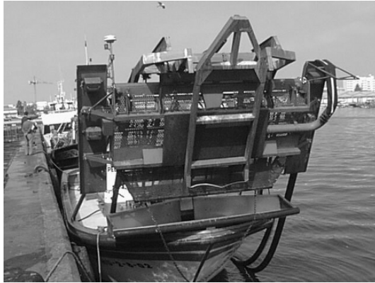
Fig. 5.4. Photograph of a hydraulic dredge used in the Chamelea gallina fishery in the southwestern coast of Spain
