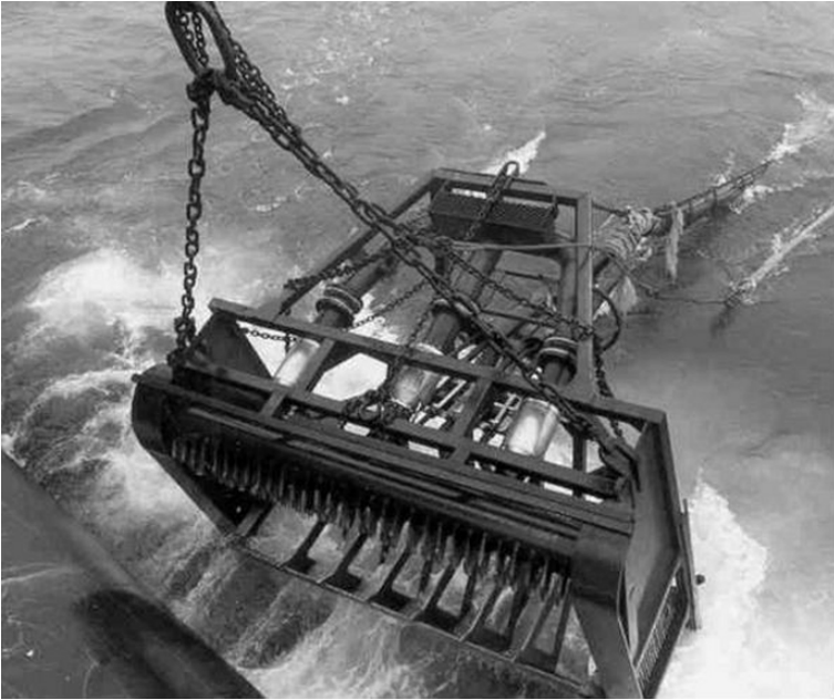
Fig. 6.5. A hydraulic dredge for surf clams in Atlantic Canada (Photo: Fisheries and Marine Institute)
