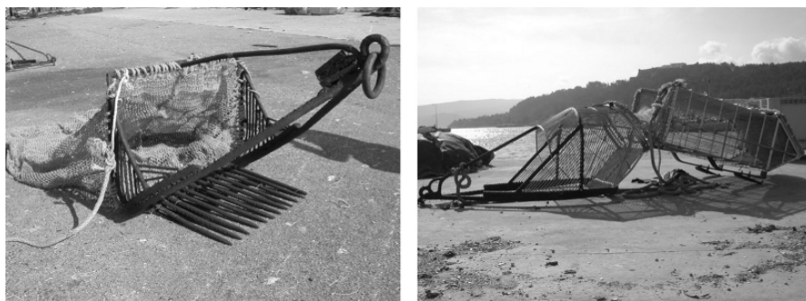
Fig. 5.3. Photographs of a razor clam dredge (left) and a clam dredge (right) used by the Portuguese dredge fleet
