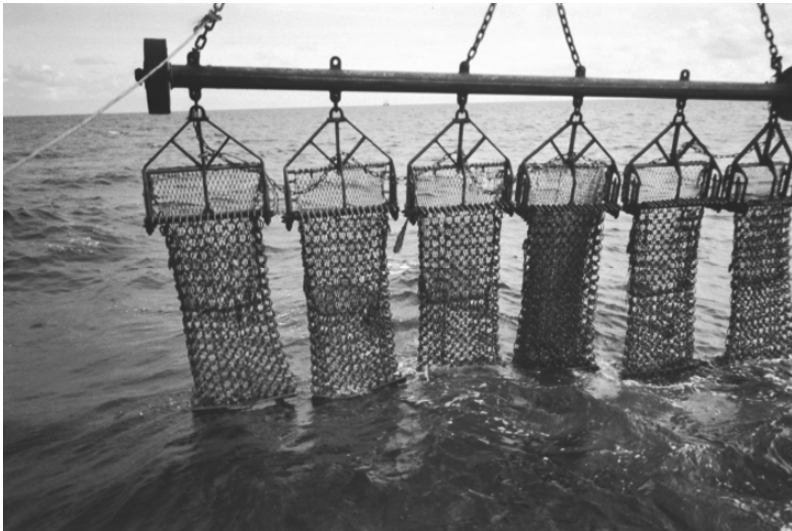
Fig. 5.2. Dredge used to harvest scallops (Photo: Antonio Hervas)
