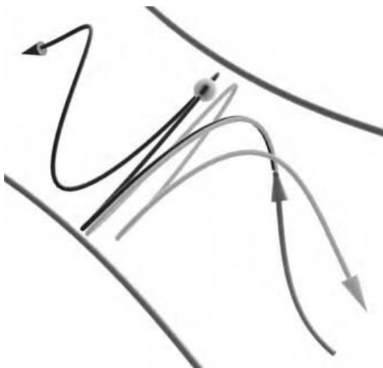
Figure 12. (The color version is available from the authors.) Two trajectories, so close in phase space that they appear as one, approach the saddle from the lower right, as in Fig. 3. After some complex dynamics around the saddle point, one reacts (crosses the TS at the dot) and goes off to the top left, and the nonreactive one returns to the lower right. We engineered this outcome by selecting their initial conditions on opposite sides of the impenetrable phase-space barrier (one of the “scissors” [20]) between reacting and nonreacting hypervolumes.
