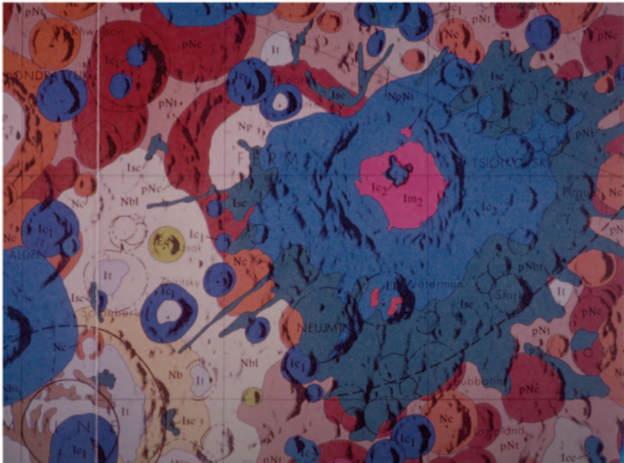
Fig. 5.38 Photo of portion of “Geologic Map of the East Side of the Moon” showing the crater Tsiolkovsky area (Wilhelms and El-Baz 1977). Ellipticity of basin (rim-to-rim) is about 0.11; asymmetry is marked by extensional features on the west (normal fault scarp) and compressional features on the eastern rim; implied directionality is WEST to EAST
