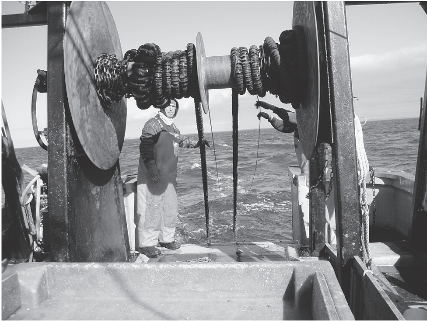
Figure 3.7. Detail of the fishing gear aboard the vessel depicted in figure 3.4 as the net is coming aboard. The round disks on the leading edge of the net, called rollers, allow the net to be dragged along the bottom, giving fishermen more access to fish and the fish less respite from fishing pressure.
