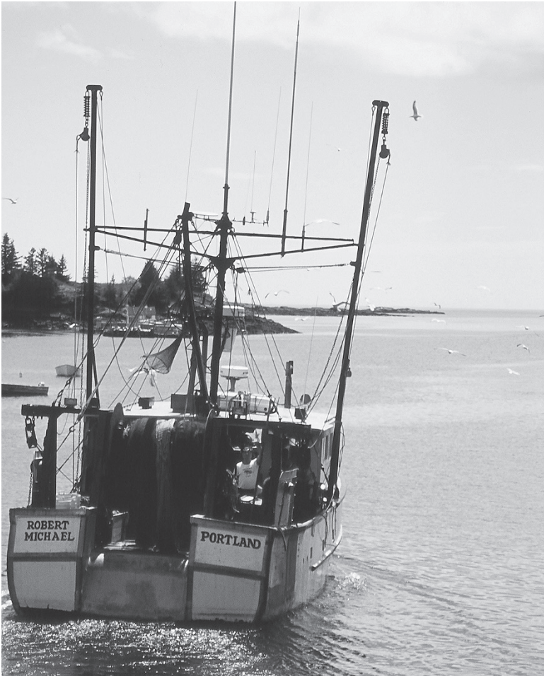
Figure 3.4. A midsize dragger (about 55 feet long) leaving port. These vessels when fishing for groundfish such as cod haul a net along the ocean floor. The elevated outriggers stabilize the boat while the net is being towed, and the drum at the rear of the boat is used to haul up or let out the net.
