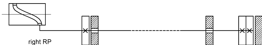
Fig. 3 Two additional repelling magnets placed into the energy accumulator at the free end
