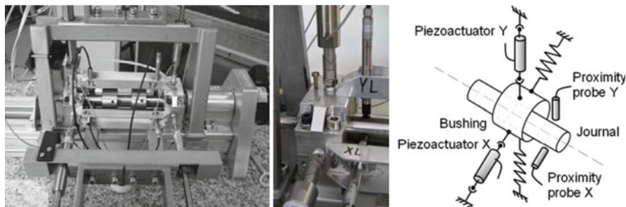
Fig. 1 Arrangement of the test rig and the controllable journal bearing
