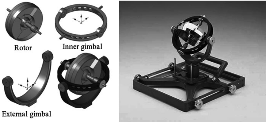
Fig. 1 Gyroscope (Phywe) and its main components
