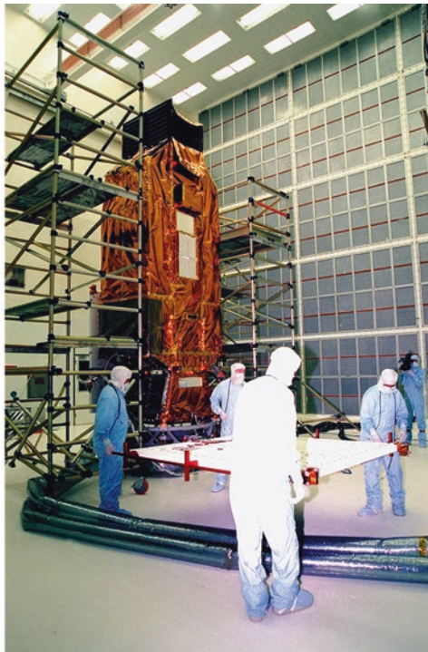
FUSE: attaching a solar panel
