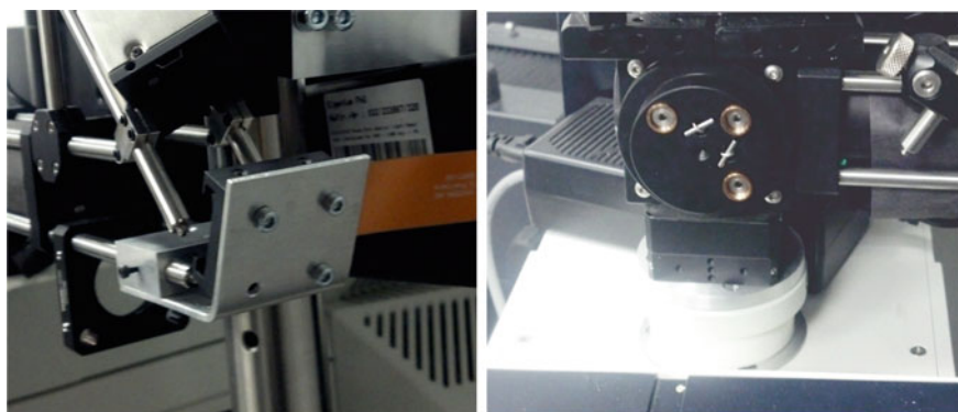
Fig. A.15 The mounting and adjustment possibilities of the spatial light modulator (left) and the dichroic mirror (right)
