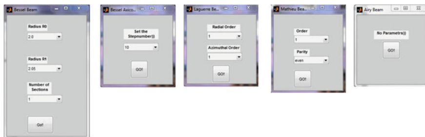
Fig. A.10 Selection window for the various beam configurations with additional parameters (from left to right: Bessel beam: OAM, Bessel beam: axicon, Laguerre, Mathieu, Airy)
