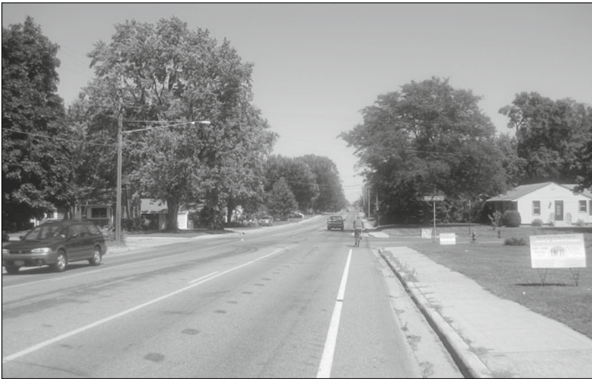
A four- to three-lane road conversion with bike lanes in Bloomington, Minnesota. (Photos by Steve Elkins.)
