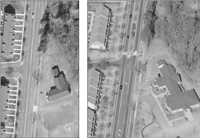
A road conversion and an improved crossing give neighborhood children in Charlotte better access to a school (at right in photo).
