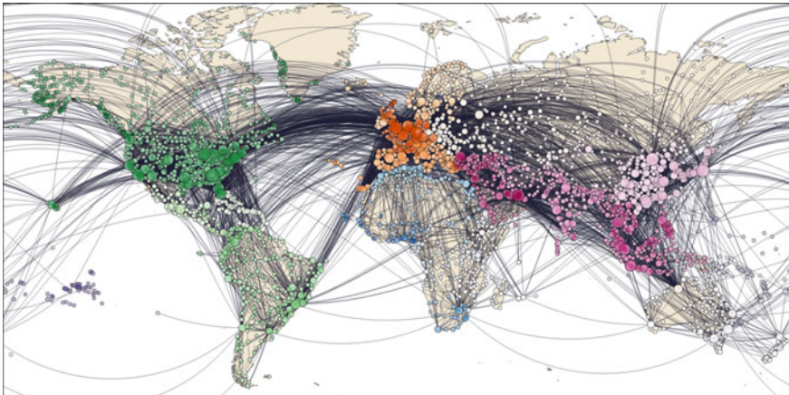
Fig. 19.1 The global air-transportation network. Each node represents one of approx. 4000 airports, each link one of approx. 50000 direct connections between airports. More than 3 billion passengers travel on this network each year. All in all every day more than 16 billion km are traversed on this network, three times the radius of our solar system
