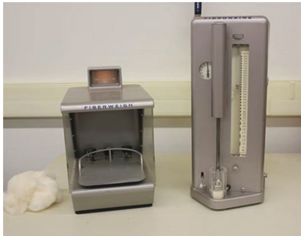
Fig. 3.20 FiberWeigh (50 grain scale) and Fibronaire testing apparatus. The Fibronaire instrument is loaded with a sample and providing a reading
