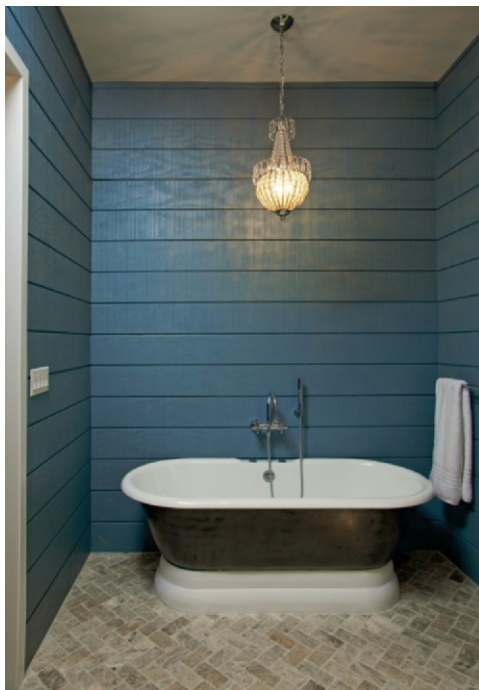
Figure 17.3 Reclaimed tub from Philadelphia, repurposed by using a Dornbracht wall-mounted faucet and handles. A new drain and stopper mechanism have been retrofitted. They are covered with basic poplar siding and have been stained. A crystal chandelier softens the atmosphere. Designed by Liz Tiesi, Threshold Interiors. Photo by Randall Bye.
