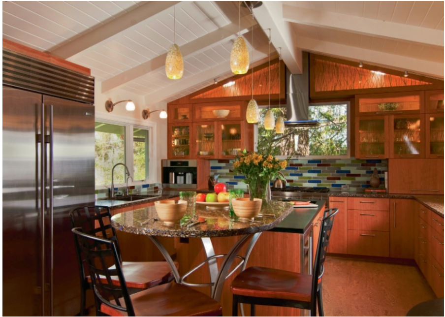
Figure 14.8 The backsplash tile is 100-percent recycled glass manufactured and sourced from base materials through finish goods within 30 miles of the project. The round raised table is Vetrazzo in charisma blue and patina color, while the rectangular portion is Paperstone in evergreen color. The cabinetry is FSC-certified, sustainably harvested cherry wood on formaldehyde-free plywood. The upper cabinet doors have 3form panels with a seaweed pattern in lieu of glass, with real seaweed sandwiched between high-recycled content acrylic panels. The cabinetry finish is OSMO Polyx-Oil, is a penetrating, plant-based finish that leaves the wood silky smooth but not shiny. The flooring is a floating cork floor from Nova Distinctive Floors in the Comprido style and sand color. The paint on the walls is a zero-VOC acrylic paint tinted with zero-VOC colorants from Yolo Colorhouse. All the lighting in the kitchen is LED.
