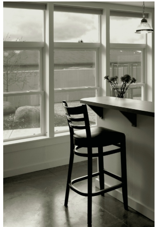
Figure 9.2 Concrete floors used to capture solar mass for radiant heating. The space also features zero-VOC paints, formaldehyde-free trim, insulated window blinds, and wheat board cabinets, and takes advantage of south-facing windows and overhangs.
