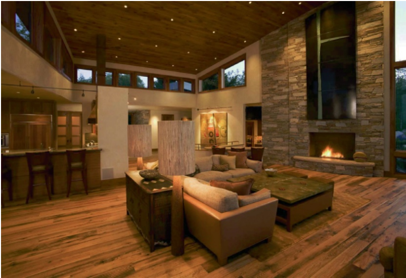
Figure 10.1 The focal point of the living space, this locally sourced stone fireplace provides thermal mass.
