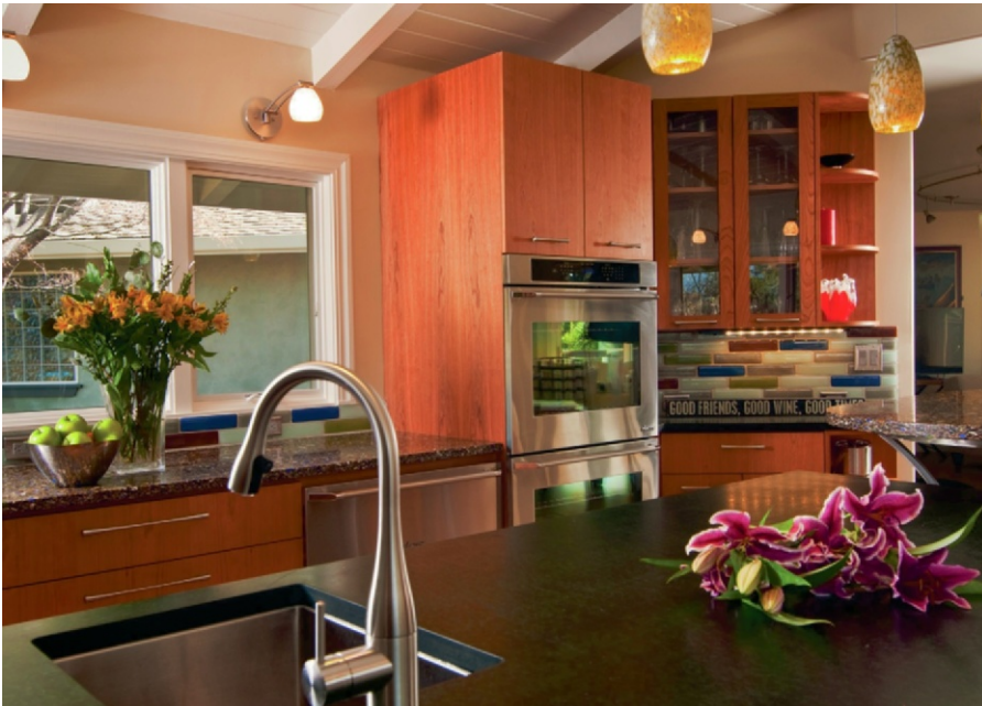
Figure 17.1 The sustainable design strategies for this kitchen included water-efficient faucets; Energy Star appliances; local, recycled glass backsplash tile; and eco-friendly cabinetry.
