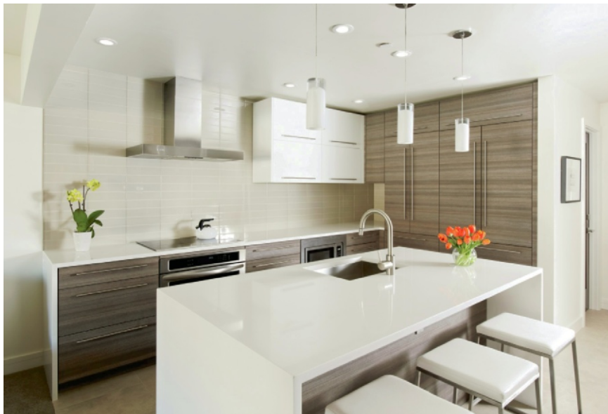
Figure 14.5 This rectangular kitchen mimics the long, narrow, rectangular shape of this open-plan living, dining, and kitchen area. The simple color scheme incorporates white quartzite countertops, stainless steel, neutral recycled content glass back splash, and gray laminate cabinetry. The floors have large-format 24-inch square commercial porcelain tiles with tight grout joints that provide a clean, neutral backdrop and high-traffic durability with slip resistance.
