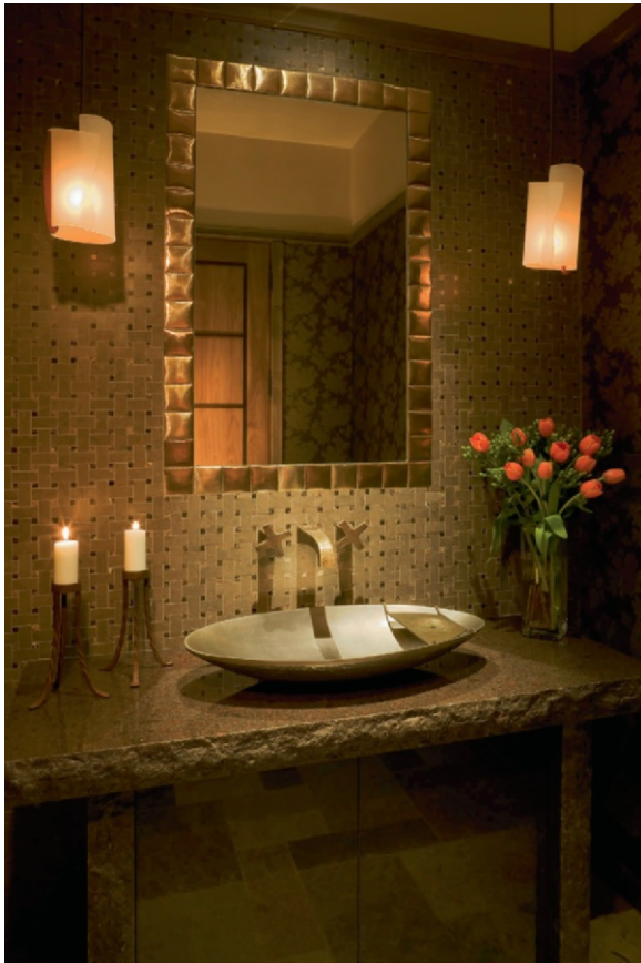
Figure 17.4 The powder room of this sustainable home includes a recycled-content metal sink, locally made bronze accent tiles, Forest Stewardship Council–certified walnut doors and trim, low-VOC substrates and adhesives, slate flooring, and compact fluorescent lamp (CFL) pendants.
