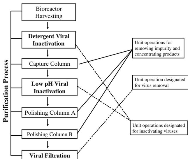
**Fig. 2** Diagram of a representative downstream purification process with multiple dedicated unit operations (in *boldface*) for viral clearance
