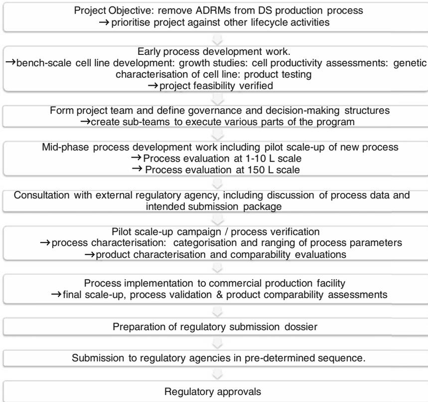
**Fig. 2** The sequence of events adopted towards project execution and regulatory approval of a major postapproval process change for production of a biopharmaceutical product
