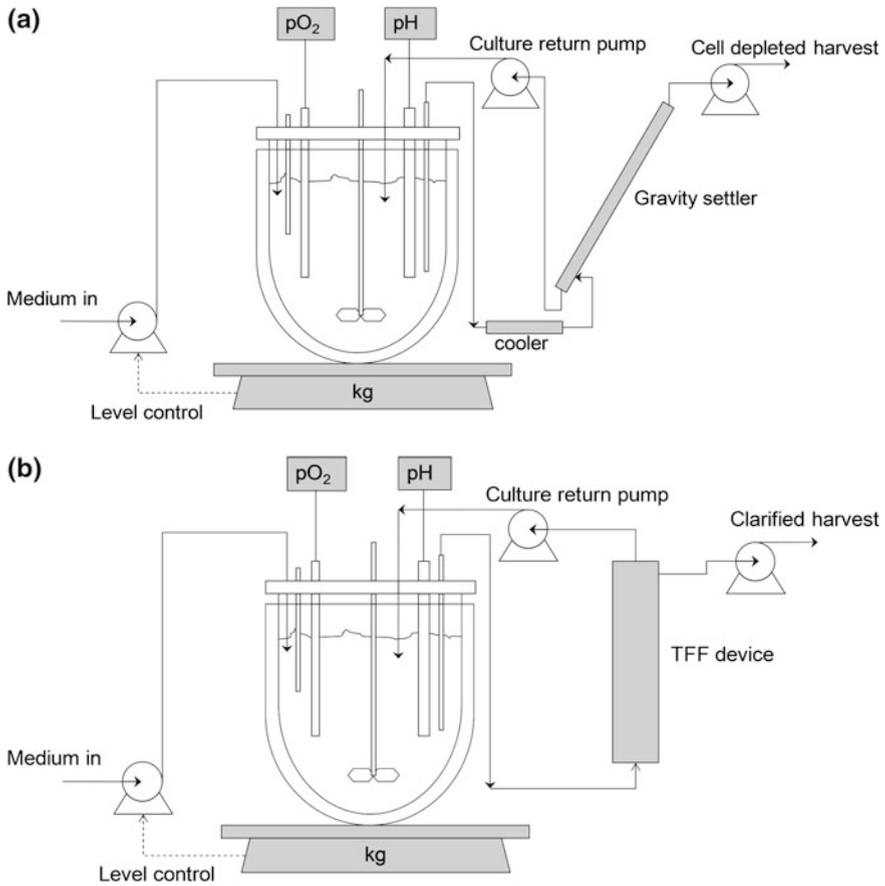
**Fig. 8** Two types of cell retention devices. Panel (a) shows a schematic of a gravity-based cell settler device and Panel (b) shows a schematic of a tangential flow filtration device
