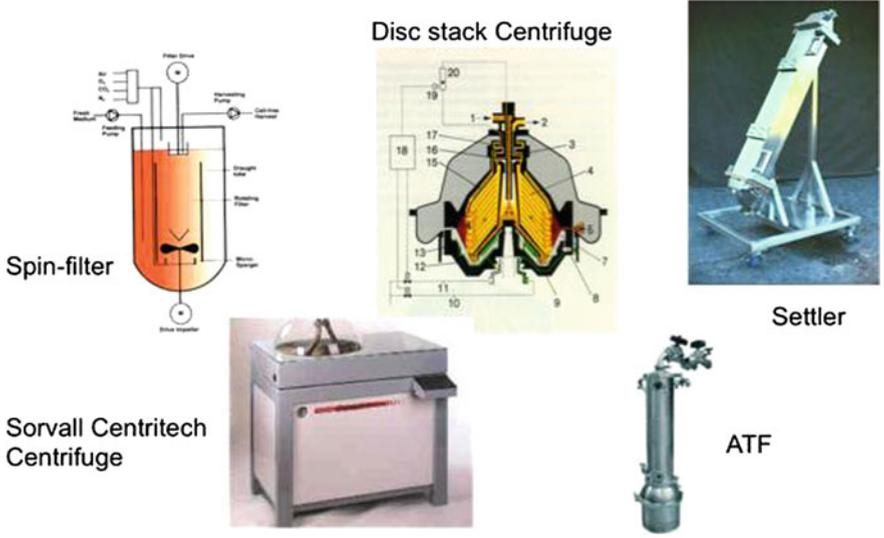
Fig. 11 Cell retention devices used for perfusion bioreactors
