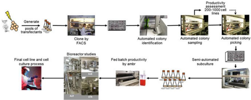
**Fig. 2** Islands of Automation. A process flow of cell culture development from transfection through to bioreactor assessment that incorporates discreet automated platforms linked together to maximize efficiency. Figure courtesy of Lonza Biologics plc
