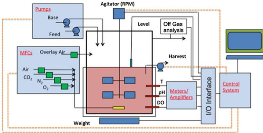
**Fig. 6** A bioreactor system with pumps, mass flow controllers (MFC), probes, meters and amplifiers, and process control units
