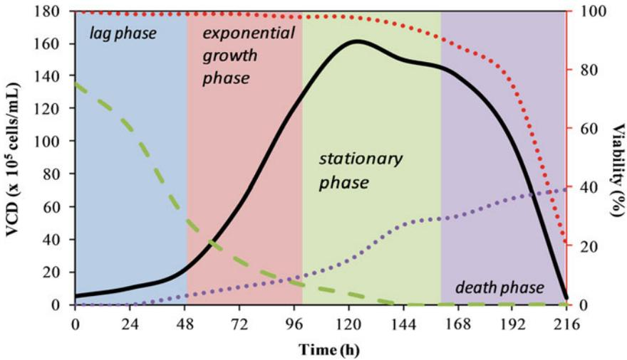
**Fig. 2** Mammalian cell growth in batch culture. *Black solid line* represents viable cell density (VCD); *red dotted line* represents cell viability; *green dashed line* represents glucose concentration in the culture; *purple small dotted line* represents product accumulation
