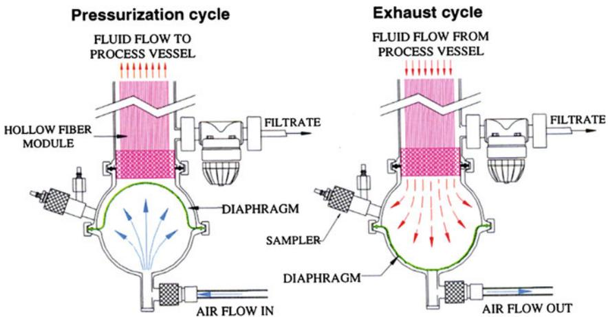
Fig. 12 Operation of alternating tangential filtration (ATF) used for cell retention [15]
