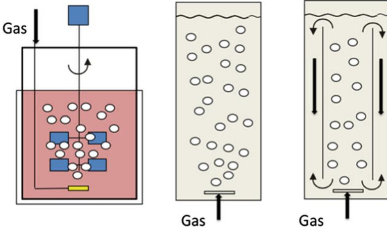
**Fig. 3** Mixing and aeration in stirred-tank (*left*), bubble-column (*middle*), and airlift bioreactor
