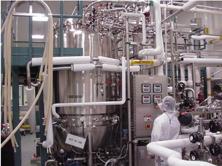
**Fig. 7** A stainless-steel bioreactor with instrumentation and piping for sterilization, gas flow, and fluid transfer
