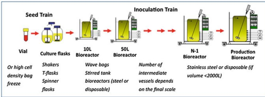
**Fig. 1** A typical upstream process used to produce biotherapeutics from cell culture
