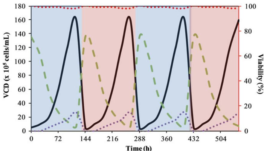
**Fig. 3** Mammalian cell growth in repeated batch mode. *Black solid line* represents viable cell density (VCD); *red dotted line* represents cell viability; *green dashed line* represents glucose concentration in the culture; *purple small dotted line* represents product accumulation
