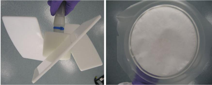
**Fig. 9** The impeller (*left*) and the Tyvec® sparger (*right*) used in ThermoFisher (HyClone) disposable bioreactors [25]
