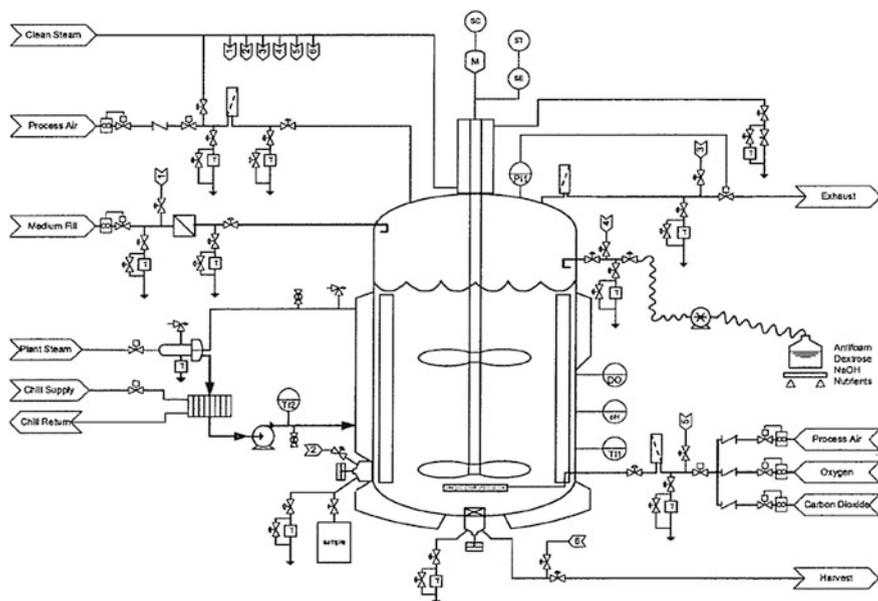
Fig. 5 Example bioreactor piping and instrumentation diagram
