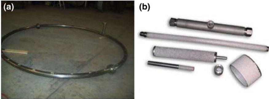
**Fig. 5** Types of spargers used in cell culture bioreactors: **a** macrosparger (arranged as a *ring* sparger), and **b** microspargers
