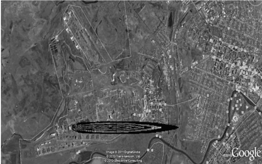
Fig. 25.13 Contaminated area (HCl, level z = 12 m, t = 20 min)
