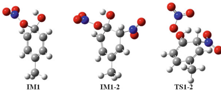
Fig. 13.2 The B3LYP/6-311 + G(d,p) optimized geometries for the addition–elimination reaction path of p -cresol where the NO 3 and NO 2 radical are added to the C1 and C2 positions. Both IM1-2 and TS1-2 are the trans conformer
