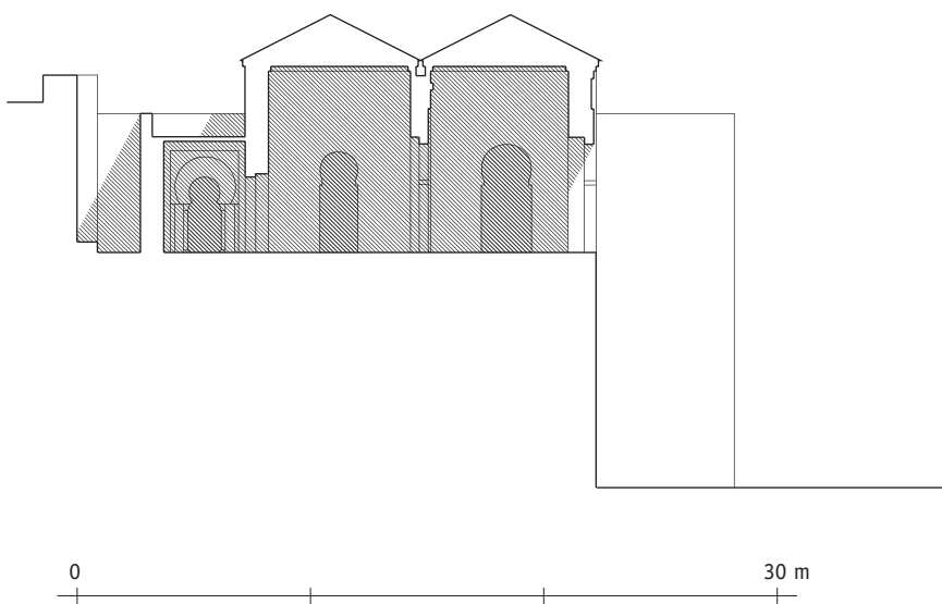
Figure 2.19 Madīnat az-Zahrā'. Reconstructed section of the Dār al-Mulk.
