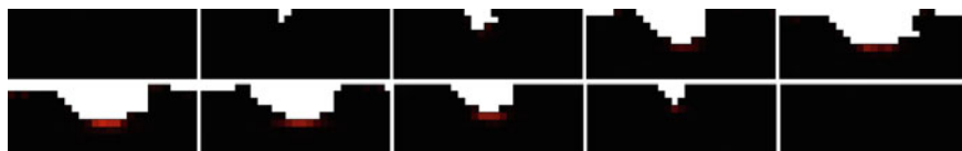
Fig. A.2 Crystallinity maps for a complete cycle (minimum strain 0%, maximum strain 70%) of NR with 40 phr N234 [#31]. The color scale is the same as in Fig. 4.27
