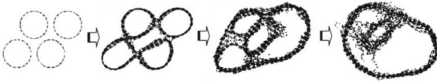
Fig. 21.2 Snapshots (top views) taken from the simulations showing the transformation of a bundle of four CNT tubes into an MWCNT consisting of two nested tubes (Reprinted with permission from Lopez et al. (2004). Copyright 2004 IEEE)
