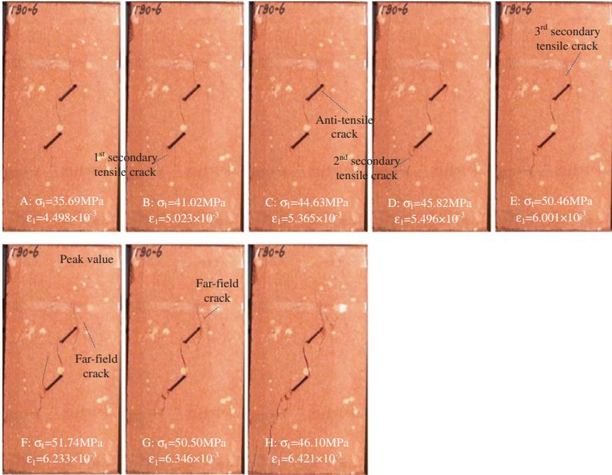
**Fig. 7.18** Fracture evolution process of red sandstone specimen T90-6# containing two parallel fissures ( $F = 600 \text{ }^\circ\text{C}$ ) after the crack coalescence between fissures ① and ② (with kind permission of Elsevier Publisher)
