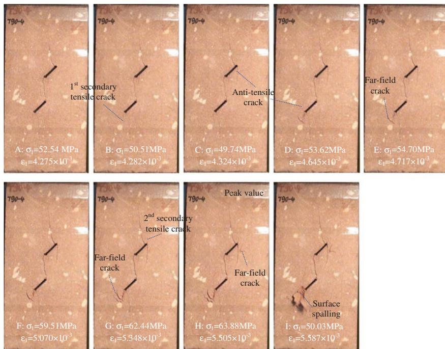
**Fig. 7.16** Fracture evolution process of red sandstone specimen T90-4<sup>#</sup> containing two parallel fissures ( $F = 300\text{ }^\circ\text{C}$ ) after the crack coalescence between fissures ① and ② (with kind permission of Elsevier Publisher)
