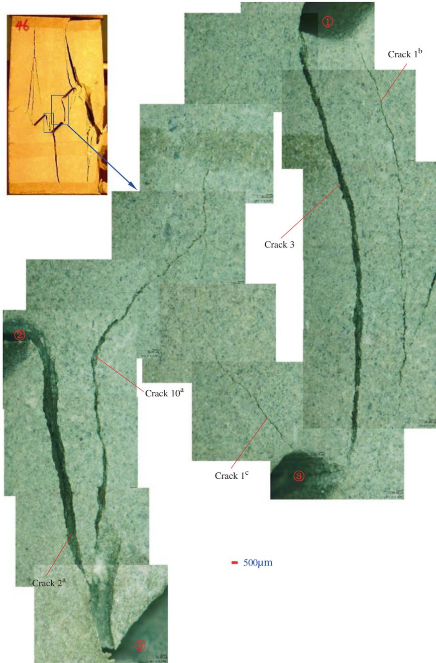
**Fig. 4.14** Microscopic observation of crack coalescence between fissures ①②③ of sandstone specimen containing three fissures ( $\alpha = \beta_1 = 45^\circ, \beta_2 = 90^\circ$ ) after failing under uniaxial compression (with kind permission of Springer Publisher)
