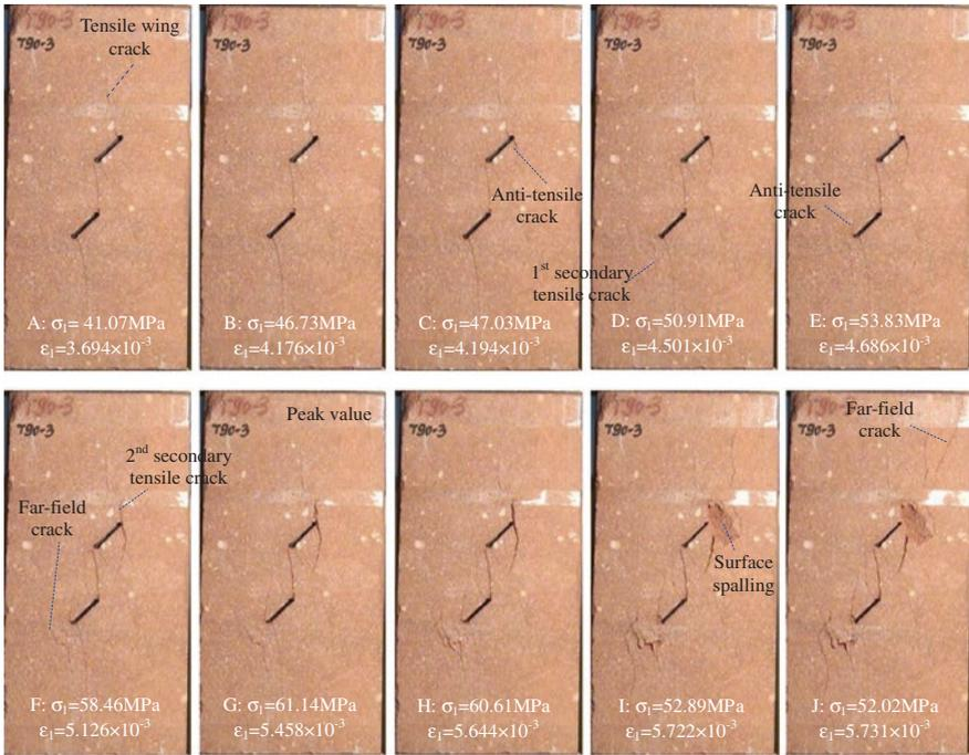
**Fig. 7.15** Fracture evolution process of red sandstone specimen T90-3<sup>#</sup> containing two parallel fissures ( $F = 300\text{ }^{\circ}\text{C}$ ) after the crack coalescence between fissures ① and ② (with kind permission of Elsevier Publisher)
