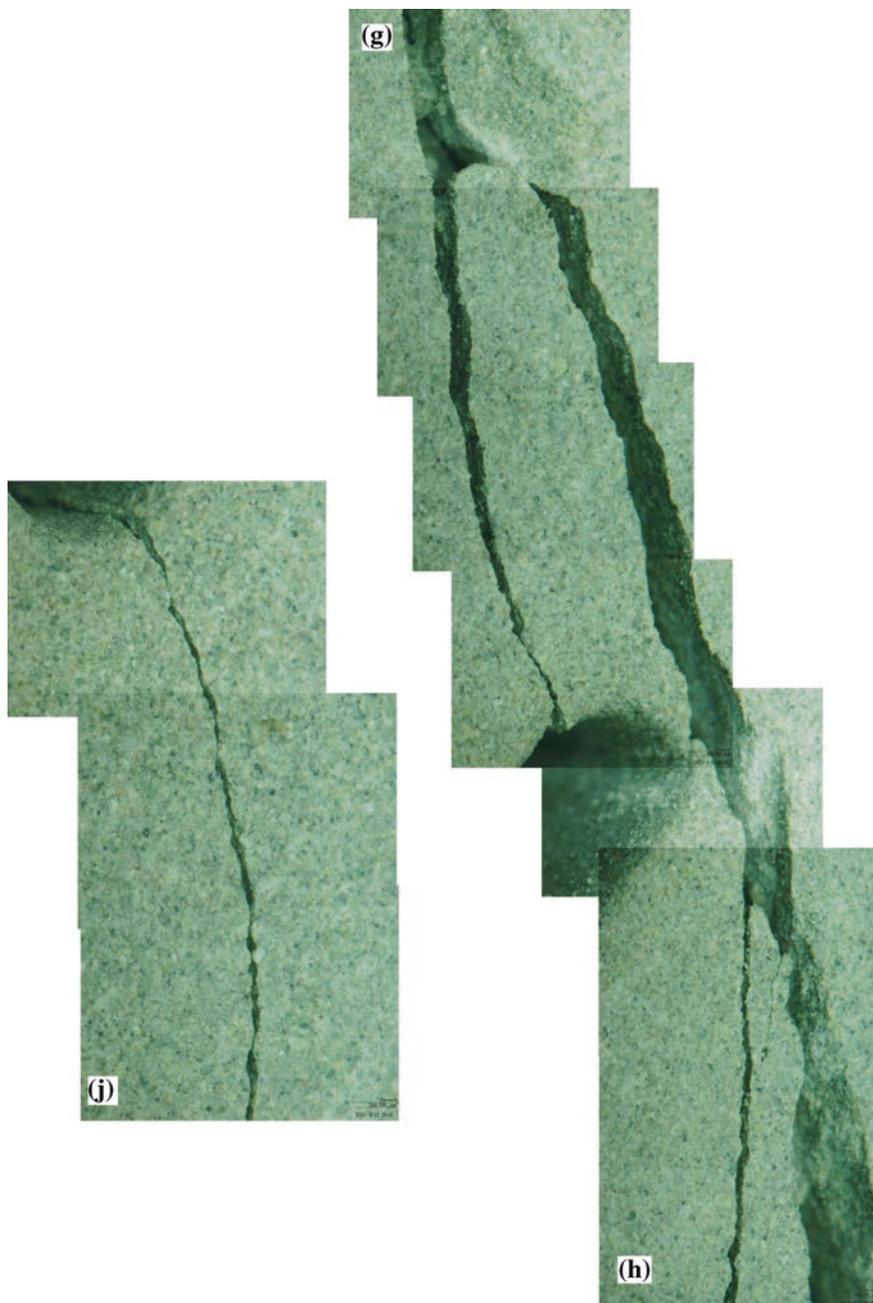
**Fig. 3.10** Local magnification of several crack coalescence of sandstone specimen containing two coplanar fissures for **g**, **h** and **j** as shown in Fig. 3.8 under uniaxial compression (with kind permission of Elsevier Publisher)
