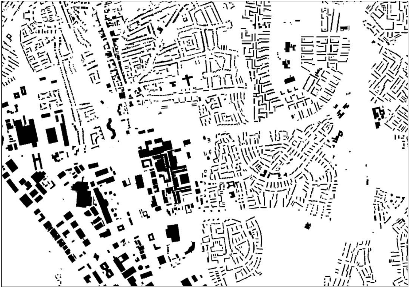
The block structure of Stevenage shows the impact of the design principles on the resulting urban form. The industrial estates are on the far left, composed of large factory structures. The town centre is next, composed of large blocks with pedestrian-only streets between them. Neighbourhood units can clearly be identified elsewhere, separated from each other by large green spaces crossed by the major road network. Stevenage Old Town can also be seen at the top left, in line with the left-hand edge of the New Town centre. Buildings fronting onto the old coaching route clearly mark out the historic urban grain.
