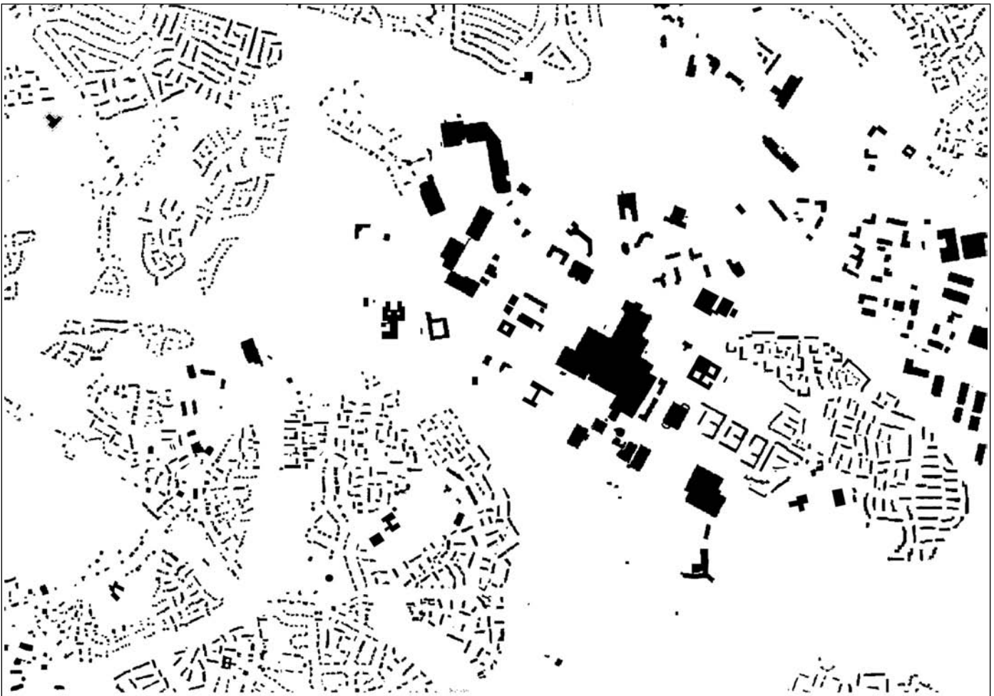
The built form of Telford shows the residential neighbourhood units and the shopping mall centre. Industrial sites are visible to the right. However, the form is more dispersed than the earlier New Towns. The empty space to the south is that formed by the town park, while that to the north of the centre is caused by the major road infrastructure of the M54.
