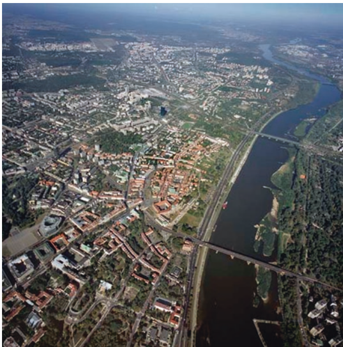
Fig. 4 Aerial photo of the Vistula River in Warsaw showing “corset” and new floodplain with the dense vegetation in the 513–514 km reach (photo by Marek Ostrowski)
