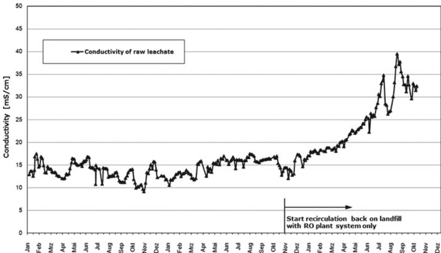
Fig. 6.13 Evolution of conductivity in the leachate after the disposal of RO concentrate back to the landfill
