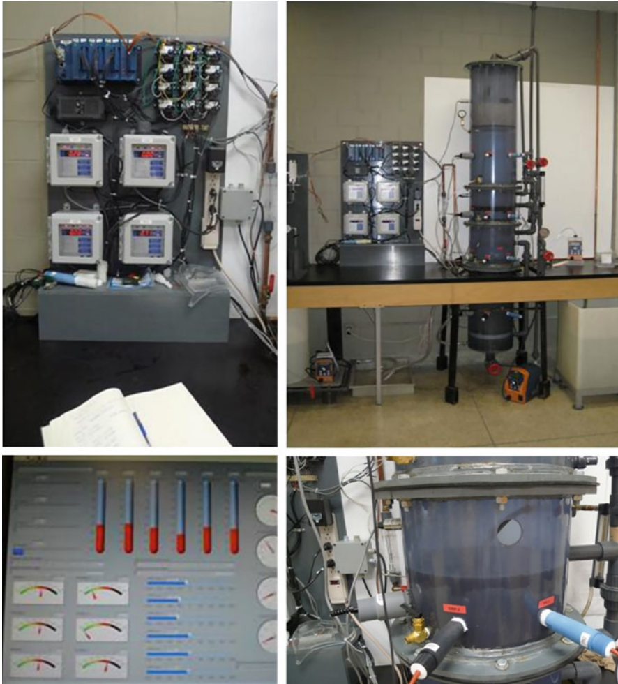
Fig. 4.8 CUBEN's pH, ORP and DO sensors connected to DAS and lab. View software
