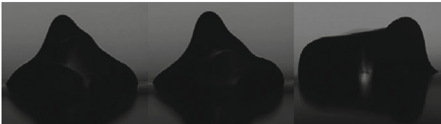
Fig. 7 Images of the side view at different instants for a 60\ \mu\text{l} drop subject to a frequency of 48 Hz, taken at a camera speed of 3,200 frames per second
