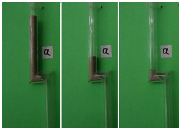
Fig. 3 Snapshots of an L-valve with \alpha = 0.98\text{ rad} and \theta_r = 0.57\text{ rad} . This valve does not maintain the granular column
