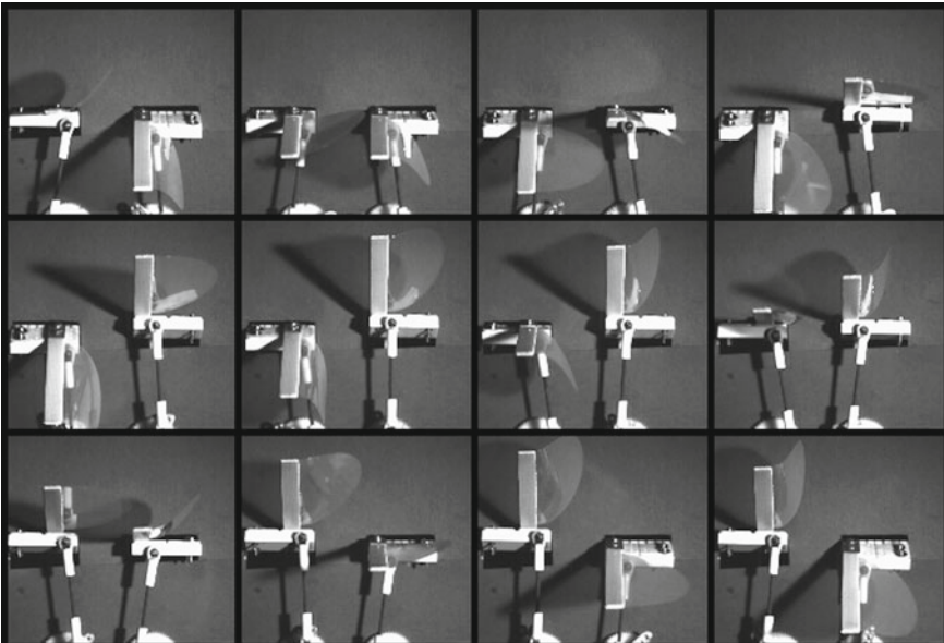
Fig. 5 Sequence showing the kinematics of the flapping wings at f = 23 \text{ Hz} and \varphi = 1.3\pi
