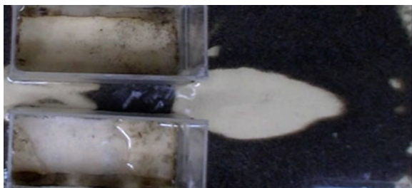
Fig. 3 Final distribution of particles in a experiment with the following conditions: H = 3 cm, f = 0.05 , Re = 1,400 , S = 0.035
