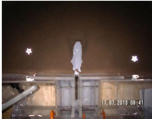
Fig. 2 Distribution of sand in the system after 15 h of forcing. The channel width is 2.5 cm and the driving period is 12.5 s. Particles concentrate inside the channel and a trough appears in front of the channel
