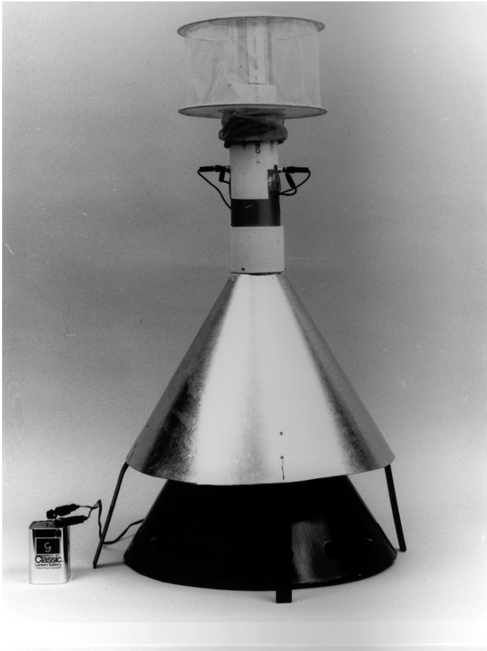
Fig. 11.4. Duplex cone trap of Freier and Francy (1991) (photograph reproduced with permission of J. E. Freier)
