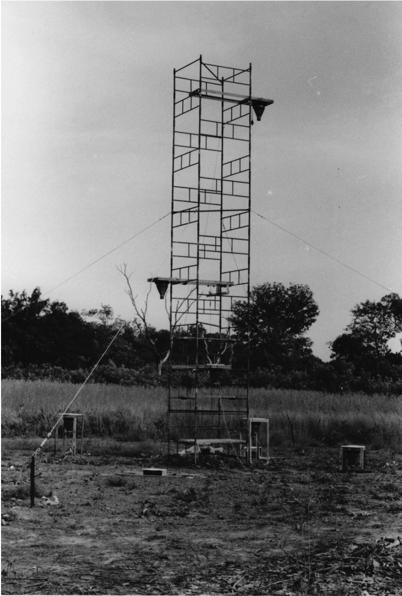
Fig. 8.4. Scaffold tower in The Gambia with Vent-Axia-type suction traps at different heights (photograph reproduced with permission of W. F. Snow)
