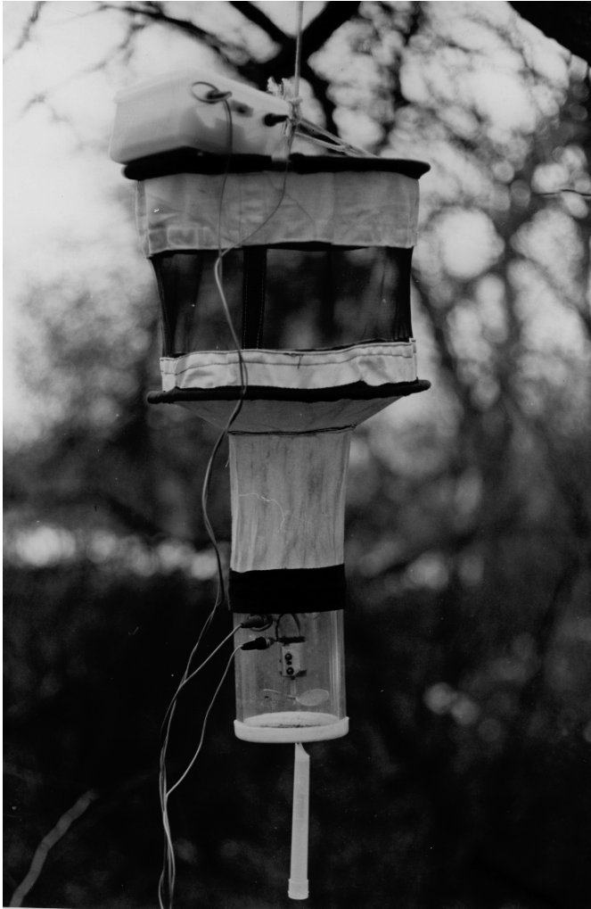
Fig. 9.16. Updraft chemical light-trap employing a light-stick (photograph reproduced with permission of M. W. Service)
