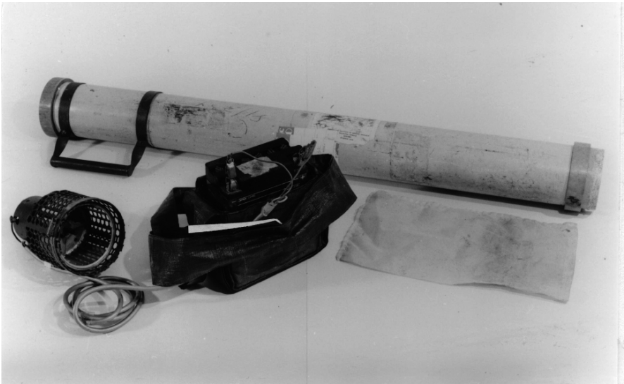
Fig. 5.21. Mechanical aspirator of Kay (1983) (photograph reproduced by permission of B.H. Kay)
