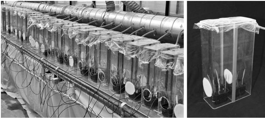
Fig. 28.2. Twin-chamber cages for the exposure of barley plants to volatile chemicals from neighbouring plants. The chambers permit only interaction via plant volatiles, while eliminating root contact and competition for water and nutrients
