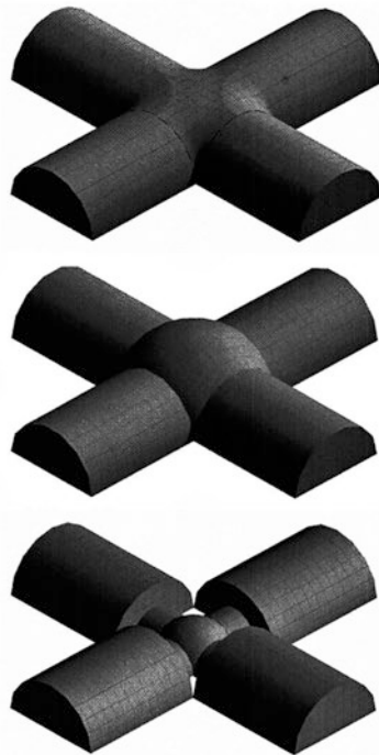
Figure 8.14. Realizations of the igloo structural concept in three possible expanded configurations. (Courtesy F. Ruess)
