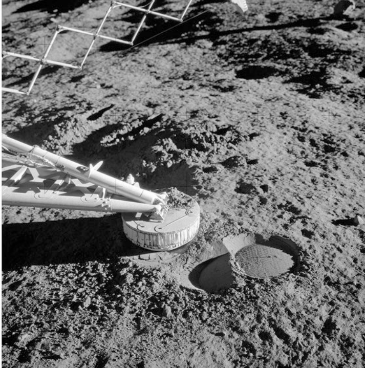
Figure 3.10. A close-up view of a footpad and surface sampler with scoop (arm, out of frame) on the Surveyor 3 spacecraft that was photographed by the Apollo 12 astronauts during their second extravehicular activity (EVA) on the Moon. The Apollo 12 Lunar Module (LM), with astronauts Charles Conrad Jr. and Alan L. Bean aboard, touched down in the Ocean of Storms only 600 feet from Surveyor 3. The television camera and several other pieces were taken from Surveyor 3 and brought back to Earth for scientific examination. The unmanned spacecraft soft-landed on the Moon on April 19, 1967. Note the extra footpad imprint in the lunar soil that was caused when the Surveyor 3 bounced upon landing. (AS12-48-7110, November 20, 1969. Courtesy: NASA)
