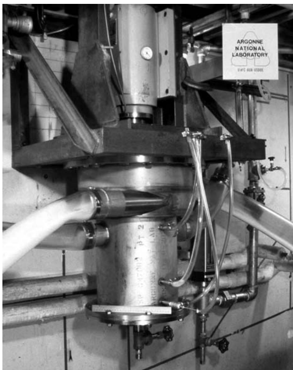
FIGURE 10.20 Operating single-stage 25-cm contactor.
