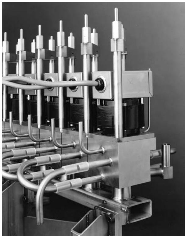
FIGURE 10.11 End of a bank of 2-cm contactors.
