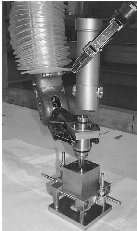
FIGURE 10.23 1.2-cm Annular centrifugal contactor by Rousselet-Robatel being assembled using remote manipulators. (Photograph was supplied by Rousselet-Robatel and is reprinted with permission.)
