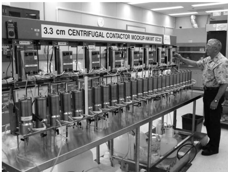
FIGURE 10.25 Twenty-six-stage 3.3-cm centrifugal contactor made of stainless steel by NIKIMT. (Photograph supplied by Jack Law and reprinted with the permission of Idaho National Laboratory (INL).)
