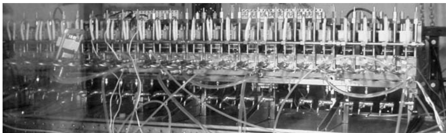
FIGURE 10.21 24-stage 2-cm centrifugal contactor in hot cell.
