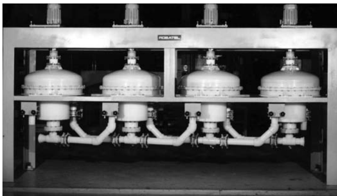
FIGURE 10.22 Four-stage 36-cm centrifugal contactor made of PVDF by Rousselet-Robatel. (Photograph was supplied by Rousselet-Robatel and is reprinted with permission.)
