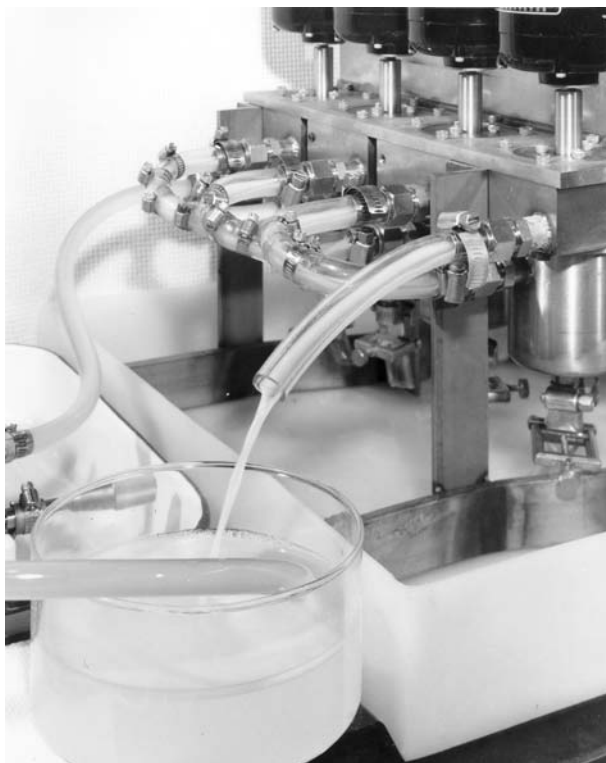
FIGURE 10.10 View of operating four-stage 4-cm contactor.
