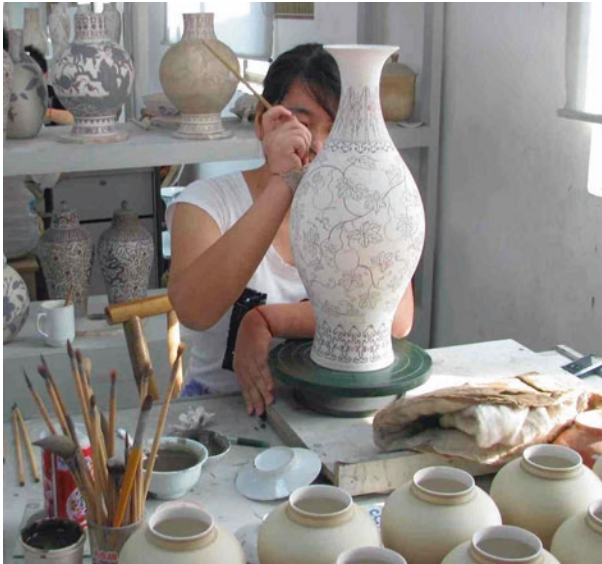
Fig. 2.2 Painter at a workshop in Jingdezhen. Note her posture and the way she uses the wheel and the paintbrush. One hand is on the wheel so that she can turn it without having to interrupt her painting. She is holding the brush in such a way as to be able to paint a certain part of the object properly depending on its curvature. Different brushes are used for different purposes, and the artisan also has to have knowledge of those. There is a small piece of sponge between the heel of her palm and the vase so that she does not smudge the parts that have already been decorated. Author photo
