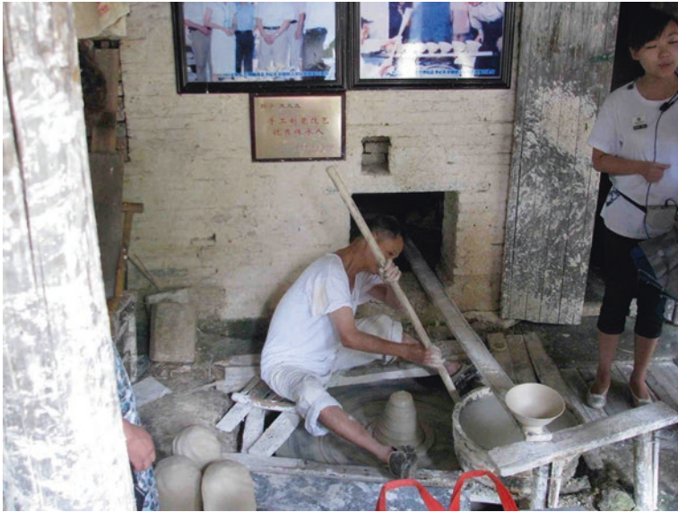
Fig. 2.3 After placing the clay on the wheel, the potter rotates it with the stick. While the wheel is moving he finishes making a bowl similar to the one on the wooden plank. According to a caption to a photograph at the Folk Kiln Museum in Jingdezhen this working posture caused the potters' bodies to change: “拉坯者因长期盘膝在坯车上劳动,致使两下肢关节 变形,走路一跨一跨,故绰号为螃蟹。” (“Because the potter works at the wheel for long periods of time with his legs bent, the joints of his lower limbs transform and he begins to walk one stride at a time, which is why he is nicknamed the ‘crab’”; translation mine.) Author photo
