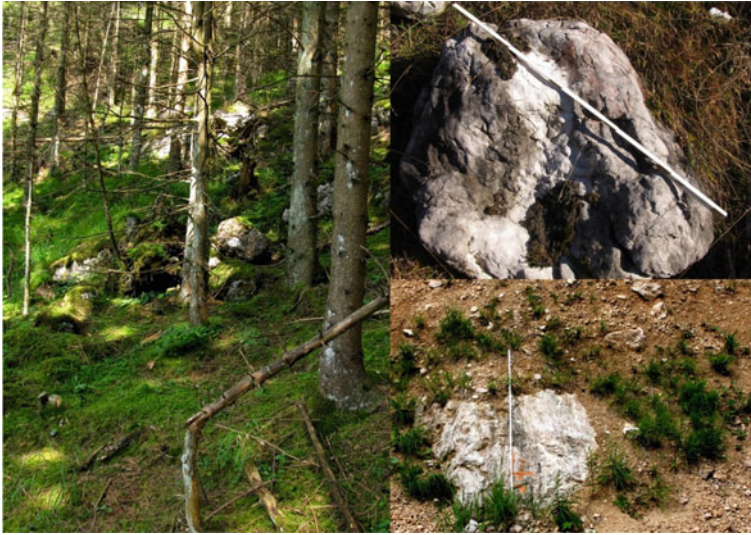
Fig. 4.11 Evaluation of block dimensions at the talus slope. Left Overview of a sample area at the mid talus slope. ( Right, Top ) Typical compact block shape of the Dachstein carbonate material. Bottom slope cut along a forest road section, exposing the talus material at the surface
