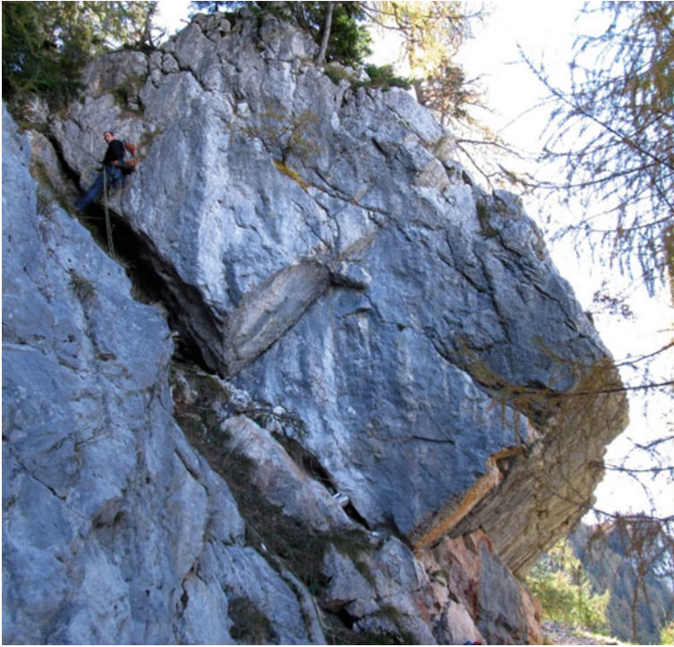
Fig. 4.1 Block at the release area, a typical example for planar failure. The block volume is approximately 200 \text{ m}^3
