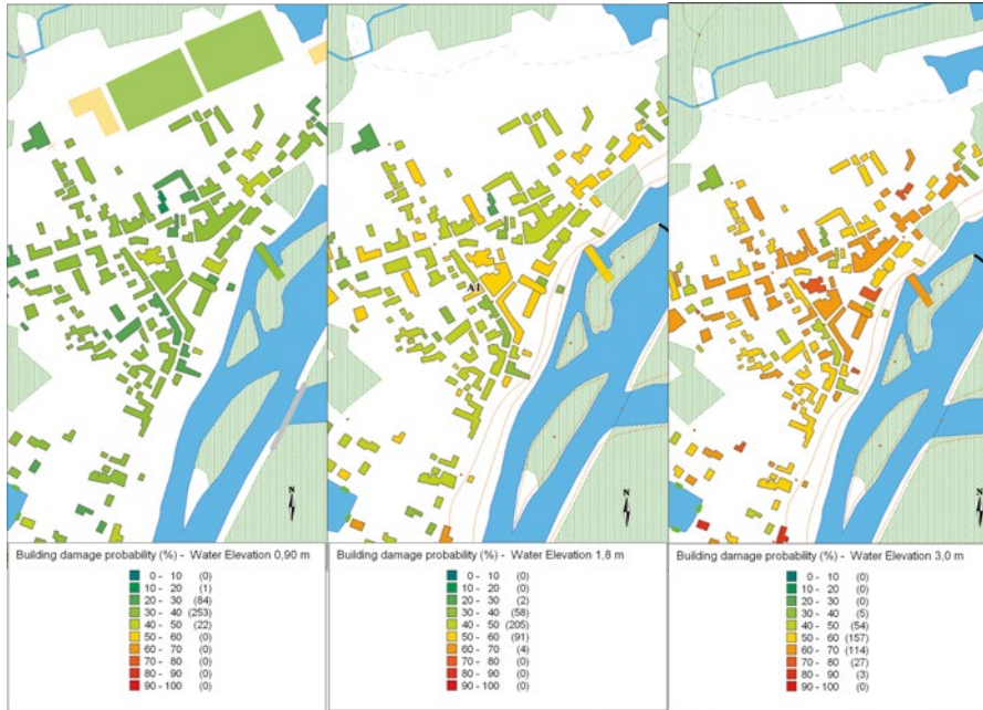
Fig. 16.5 Risk maps: evolution of damage failure in buildings at three different levels of flooding (Source: Mebarki et al. 2012; in Nat. Hazards Earth Syst. Sci)
