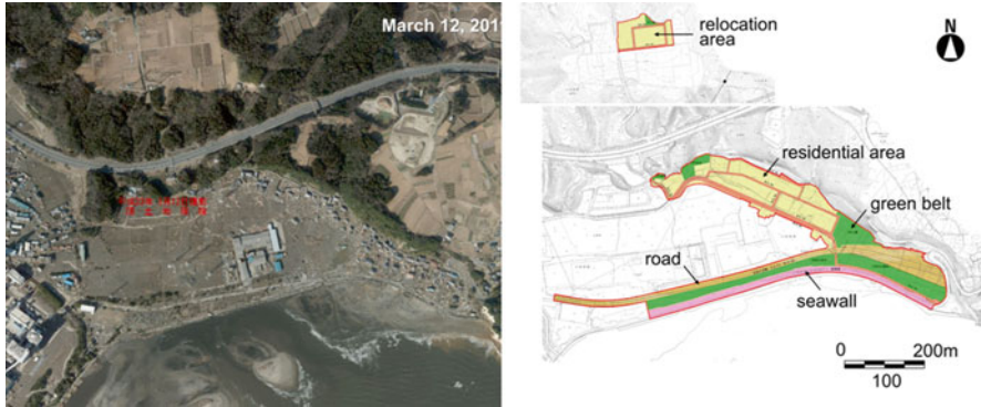
Fig. 13.17 Reconstruction Plan of the Iwama District, Iwaki City, as compared with a post-tsunami aerial photograph
