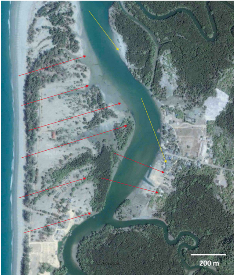
Fig. 6.3 Directions of the tsunami wave hitting the Andaman Coastal Research Station for Development, the Nua and the Hat Sai Khao villages. Note that the tsunami wave travelled both across the Praphat beach (indicated by the red arrows ) and along the distributary channel, the Kamphuan canal (indicated by the yellow arrows ) (Source: Google Earth (2/6/2005))
