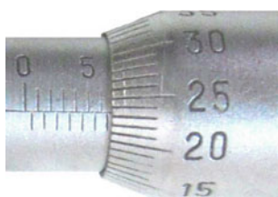
Fig. 1.9 Reading a micrometer (II). The nearest sleeve division to the edge of the thimble is the 6.5 mm division. The thimble division lies almost in the middle between the 23rd and 24th divisions, so we may take 23.5 as the closest division. The micrometer reading is therefore 6.5 + (23.5 \times 0.01) = 6.735 mm
