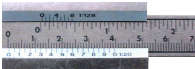
Fig. 1.7 Positive zero correction. Note that the zero of both the top (inches) and lower (millimetres/centimetres) Vernier scale is to the right of the zeros of the main scale. Since the 8th division on the Vernier scale is aligned with a division on the main scale, the positive zero correction to be subtracted from the Vernier caliper reading is (8 \times 0.05) = 0.4 \text{ mm}
