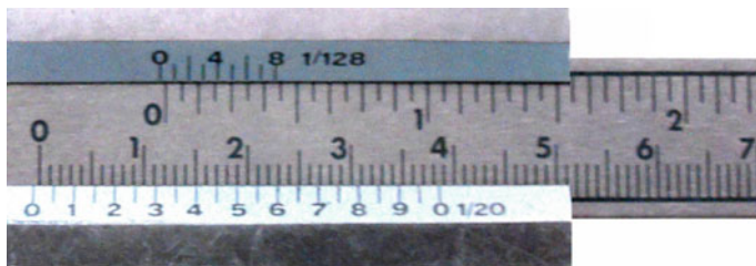
Fig. 1.6 Negative zero correction. Note that the zero of both the top (inches) and lower (millimetres/centimetres) Vernier scale is to the left of the zeros of the main scale. Since the 8th division on the Vernier scale is aligned with a division on the main scale, the negative zero correction to be added to the Vernier caliper reading is (8 \times 0.05) = 0.4 \text{ mm}
