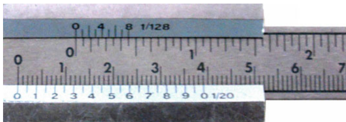
Fig. 1.4 The figure shows 20 divisions of the Vernier scale covering 39mm of the lower main scale, so that the divisions of the Vernier scale are each 1.95 mm long
