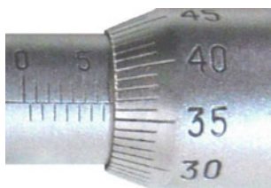
Fig. 1.8 Reading a micrometer (I). The nearest sleeve division to the edge of the thimble is the 7 mm division. The thimble division most closely aligned with the reference line is the 37th division. The micrometer reading is therefore 7 + (37 \times 0.01) = 7.37 mm
