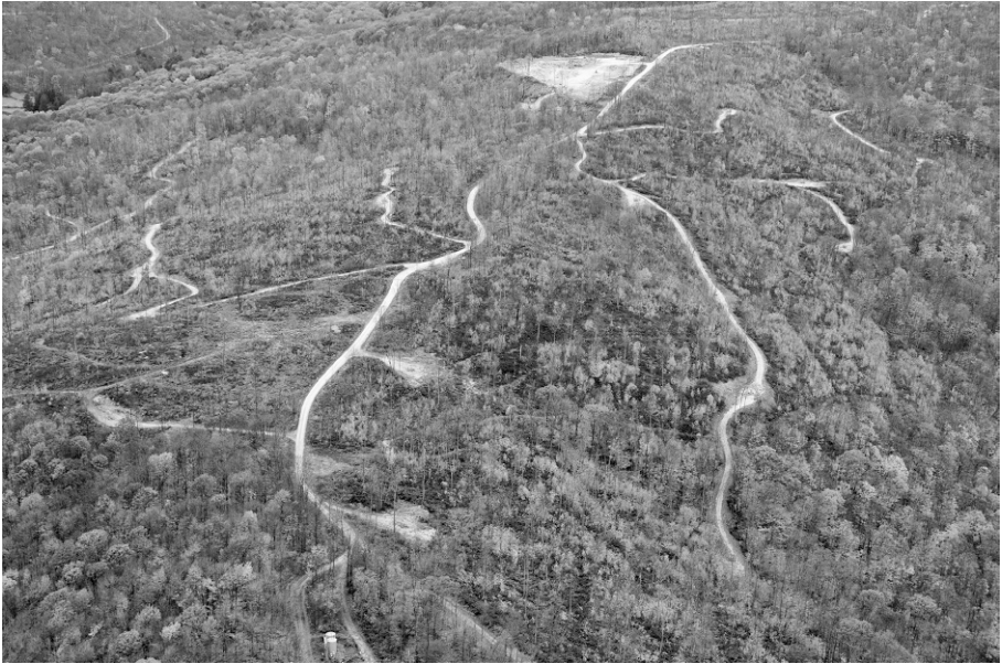
Figure 12.1 Roads in the Allegheny National Forest in Pennsylvania. The U.S. Forest Service estimated in 2011 that oil and gas companies had built 2,083 miles of roads within this forest. These roads exist in addition to another 1,243 roads used for timber harvesting and administration. The roads cause habitat fragmentation for wildlife and vegetation. © Carl Heilman II/Wild Visions, Inc. with flight support from LightHawk.
