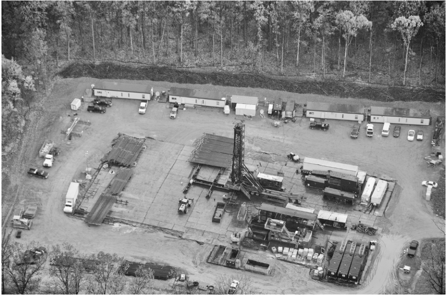
Figure 12.4 Marcellus Shale well drilling in Elk State Forest, Pennsylvania. Shale oil drilling uses heavy equipment, requiring the clearing of up to five acres of forestland. In addition, each fracturing operation draws between five million and six million gallons of water from forest rivers and streams. © Carl Heilman II/Wild Visions, Inc. with flight support from LightHawk.
