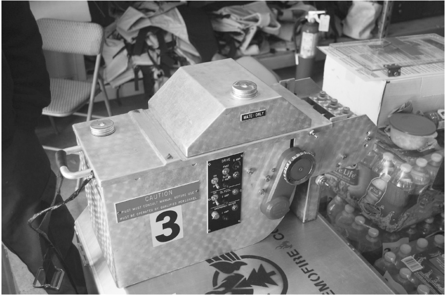
Figure 8.2 Premo MK III Plastic Sphere Dispenser. Pilots fly helicopters over an area of Florida's national forests scheduled for a prescribed burn, and fire officers dispense plastic spheres from this dispenser. The spheres ignite and set small fires, which are controlled by officers on the ground. Photograph by Christopher Johnson.
