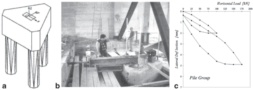
Fig. 11 Horizontal loading test on pile group. a Piles scheme. b View. c Loading test results
