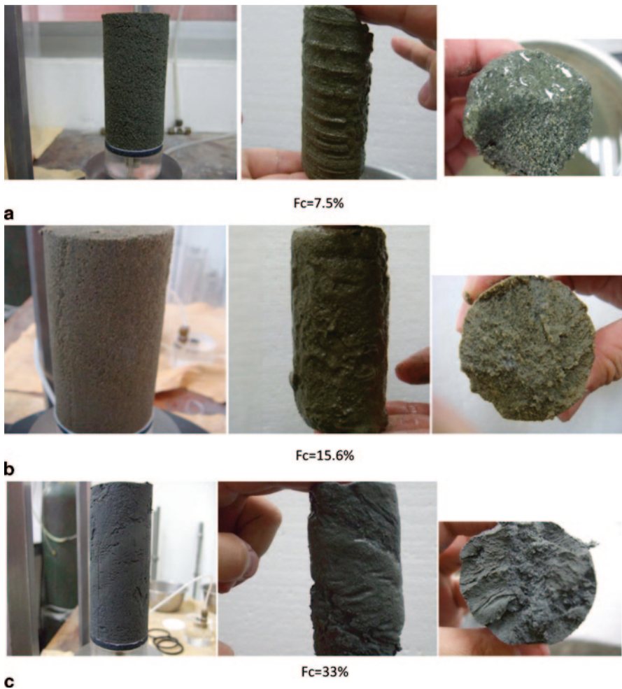
Fig. 9 Undisturbed non-plastic silty sand specimens retrieved using Gel-Push sampling technique (before testing, after testing, and cross section)
