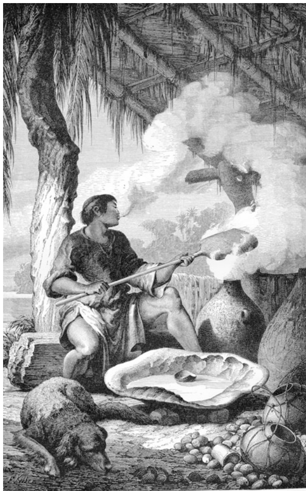
Fig. 14.8 Rubber tapper smoking latex over a fire using fruits of Attalea phalerata for fuel in the second half of the nineteenth century. The tapper periodically adds a fresh layer of latex scooped from the carapace of a giant river turtle ( Podocnemis expansa ). Madeira River, Brazil (Keller 1874: 101)
