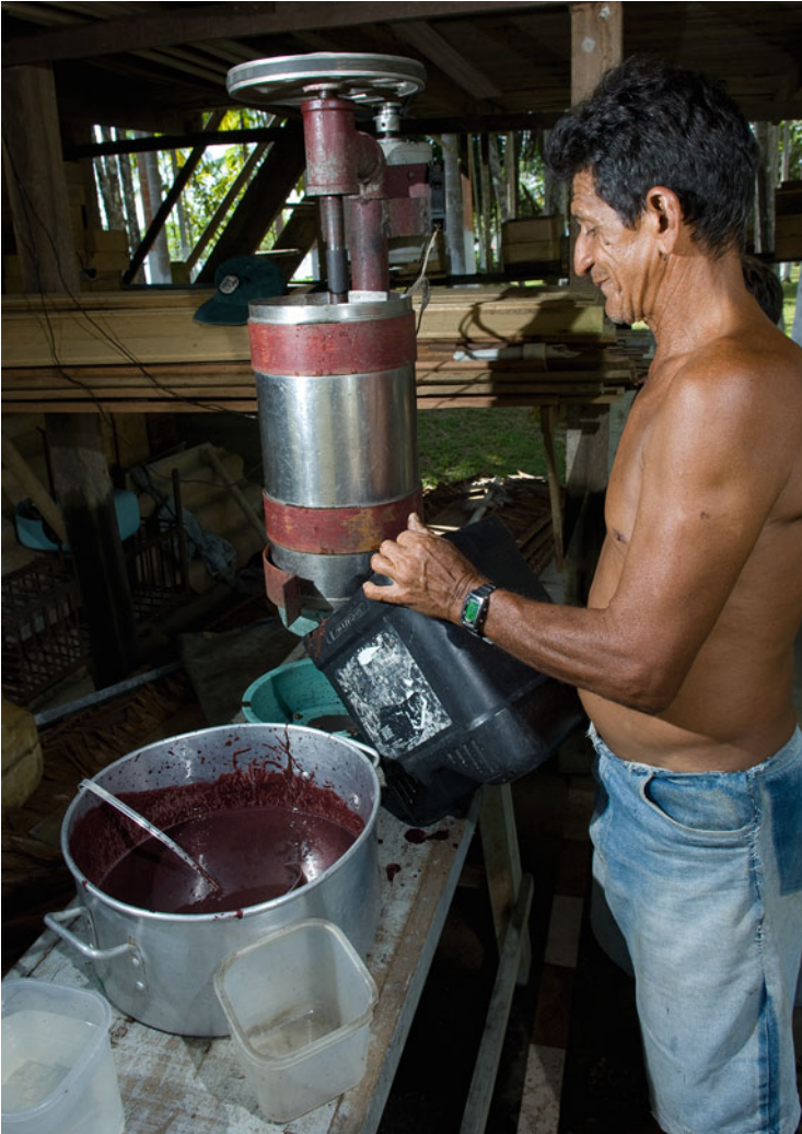
Fig. 35.3 Electric beater ( batideira ) for making juice from açai ( Euterpe precatoria ) fruits. Lago Miwá near Codajás, Solimões River, Amazonas, Brazil, 6-24-07
