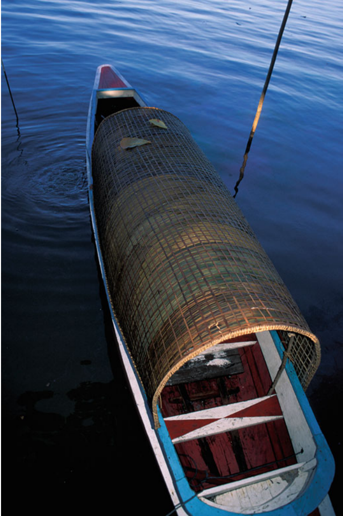
Fig. 45.3 Buçú ( Manicaria saccifera ) thatch on a motorized canoe ( rabeta ). The fronds have been laid over a framework of split petioles of arumã ( Ischnosiphon obliquus ). Afuá, Marajó Island, Pará, Brazil, 8-16-98
