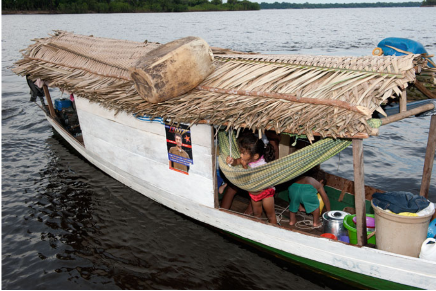
Fig. 15.3 River boat thatched with Attalea racemosa fronds and powered by a small outboard motor ( rabeta ). Confluence of the Jaú and Negro Rivers, Amazonas, Brazil, 10-4-12
