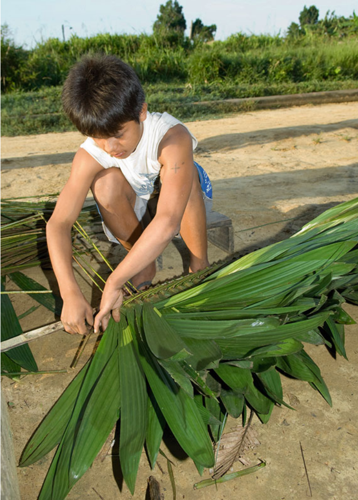
Fig. 44.1 Pleating leaflets of irapay ( Lepidocaryum tenue var. tenue ) over a pole cut from the trunk of pona ( Socratea exorrhiza ) palm. After drying, the panels of folded irapay fronds will be used for thatch. Jenaro Herrera, Ucayali River, Loreto, Peru, 1-11-06
