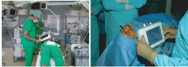
FIGURE 16.14 Display options that direct the view at the patient. Left: semitransparent LCD mounted on a swivel arm. Right: tracked LCD with a camera on the other side. (Left image courtesy BERND SCHWALD of the MEDARPA project, ZGDV Darmstadt; right image courtesy TIM LUETH and STEFAN WEBER, MiMed, University of Technology München)
