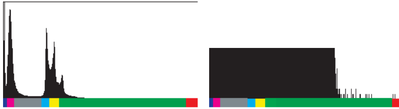
FIGURE 6.2 Left: linear histogram. Right: vertical zoom into the bottom end (frequencies 0–10) of the linear histogram. The linear horizontal scale is inappropriate for the histogram of this CT dataset of a human thorax, since the large majority of voxel values is concentrated on the left side. A vertical zoom can provide more information on the upper voxel values. The colored rectangle on the bottom marks the different materials in the intensity value spectrum. The respective classification can be found in Figure 6.4 (right).
