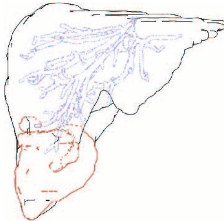
FIGURE 17.21 Hidden feature lines are rendered as dashed lines. With this technique, additional information concerning a tumor and the intrahepatic vasculature are included in a visualization. (Image courtesy ANGELA BRENNER, University of Magdeburg)
