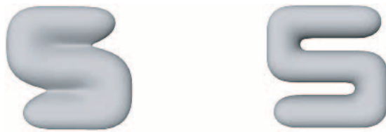
FIGURE 14.27 Distance between the branches of the S-shapes is 3 mm. The radius of all branches is 1.37 mm. Unwanted blending (left) is considerably reduced with the narrower filter (right) [OELTZE and PREIM 2005]. (Images courtesy STEFFEN OELTZE, University of Magdeburg)
