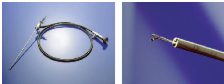
FIGURE 15.1 Neuroendoscope with one working channel. Left: neuroendoscope; left is the trochar that guides the actual endoscopic optic (right) to the target area. On the right side is the ocular, which is used to acquire the endoscopic image. Right: endoscope with one working channel containing a plier. (Images courtesy FRANK DUFFNER, University of Tübingen)
