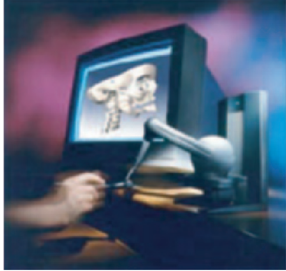
FIGURE 12.10 Cut boundary specification with a tactile input device (Phantom, SensAble Technologies). (Image courtesy STEFAN ZACHOW, Zuse-Institute Berlin)
