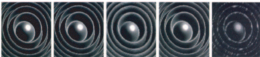
FIGURE 9.36 Different renditions of the Marschner-Lobb phantom. The three leftmost images and the rightmost image are created with standard ray casting, whereas the next image (second from the right) was generated with a coherent projection approach. The rightmost image is created with ray casting using a preclassified volume rendering pipeline. All images are generated with trilinear interpolation, except the middle image, which employed a cubic interpolation filter [KIM et al. 2001]. (Images courtesy KWANSIK KIM, University of California, Santa Cruz)
