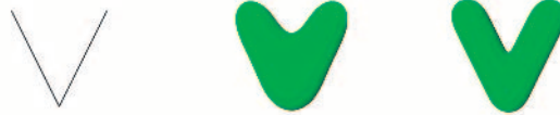
FIGURE 14.23 Blending strength, left: skeleton; middle: high blending strength; right: reduced blending strength [OELTZE and PREIM 2005]. (Images courtesy STEFFEN OELTZE, University of Magdeburg)
