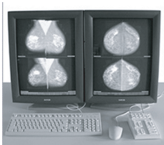
FIGURE 4.4 Soft-copy reading of digital mammograms. The two vertical monitors support comparisons between the current images and previous images. The keypad on the right provides access to the most important functions, such as changes of the layout. (Image courtesy MeVis BreastCare, Bremen)
