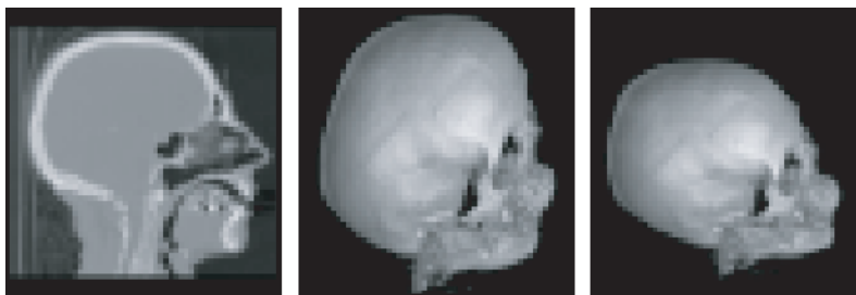
FIGURE 9.9 Shear warp planes. From left to right: Volume slice, base-plane image; final (image-plane) image [LACROUTE 1995]. (Images courtesy PHILIPP LACROUTE)
