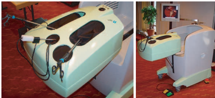
FIGURE 20.36 The Virtual Endoscopic Surgery Training (VEST) system “VSOne” and its realistic haptic interface. Left: an overview with a display that resembles the “real” endoscopic view. Right: detailed display of the haptic surgical devices. (Image courtesy HÜSEYİN ÇAKMAK, Forschungszentrum Karlsruhe and Select-IT VEST Systems AG)
