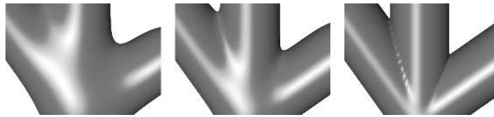
FIGURE 14.36 Influence of varying \omega on the blending strength at branchings. The close-ups of the trifurcation from Figure 14.26 were generated using \omega = 2 \ln 2 , \omega = 5 \ln 2 , and \omega = 30 \ln 2 (from left to right). With \omega = 2 \ln 2 , the blending strength is barely reduced. Using \omega = 30 \ln 2 the surface exhibits creases at the skeleton joint [OELTZE and PREIM 2005]. (Images courtesy STEFFEN OELTZE, University of Magdeburg)
