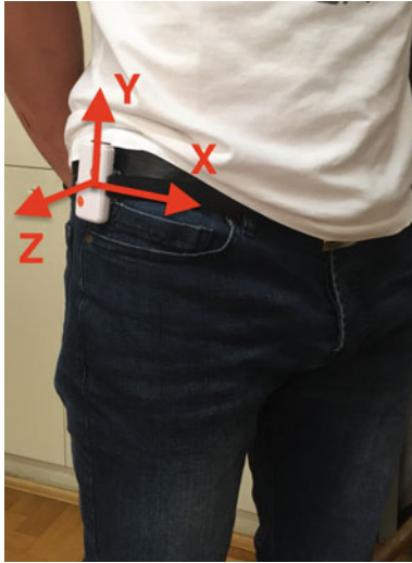
Fig. 1 Sensor placement—Y axis was pointing up (vertical), X axis was pointing forward (antero-posterior plane) and Z axis was pointing away from the body (medio-lateral plane)
