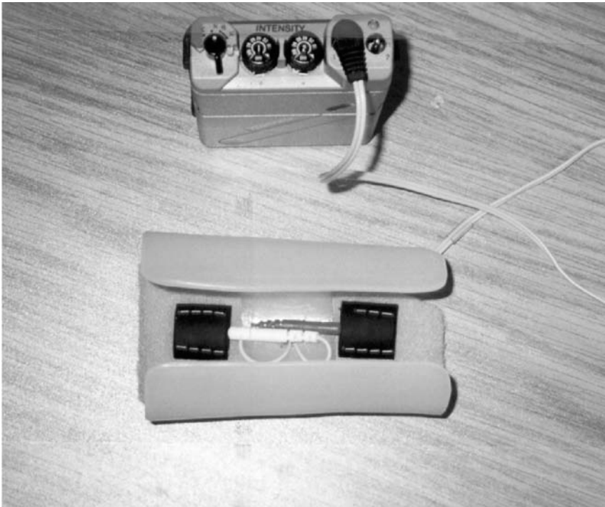
Figure 5.2 An electrical stimulator connected to a right wrist electrode cuff.
