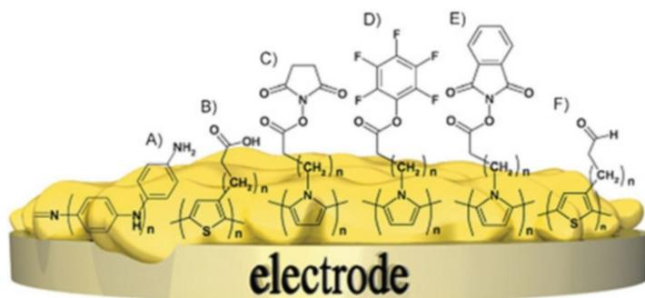
**Fig. 2.14** Examples of functionalized polymer films bearing reactive groups for covalent anchoring of biomolecules. (A) amines (PANI), (B) carboxyls (PTh), (C) *N*-hydroxysuccinimide esters (PPy), (D) pentafluorophenyl esters (PPy), (E) *N*-hydroxy-phthalimide esters (PPy), (F) aldehydes (PTh) (Reprinted from Ref. [144] with the permission of Royal Society of Chemistry)
