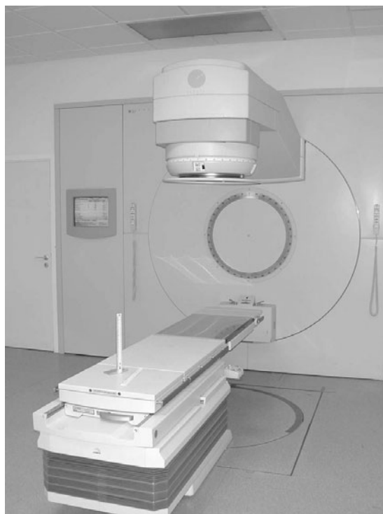
Figure 25.1 A linear accelerator.
