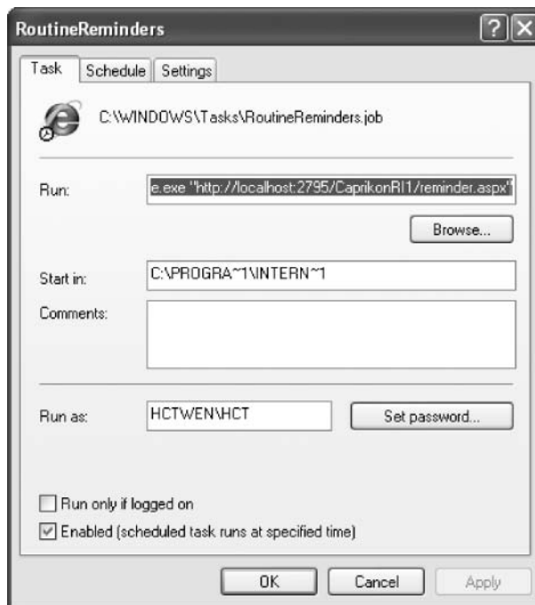
Figure 6.6 Configure the 'Scheduled Tasks' to execute the email script
