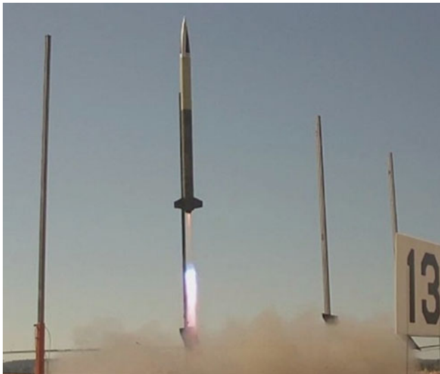
Fig. 1.8. Liftoff of a model rocket. During the first 2 m of its journey it moved up the metal post. This helped it move upwards (Credit: Chris Keir).
