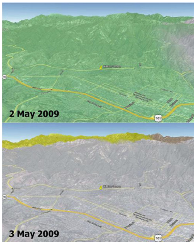
Fig. 3.4. This image shows the soil moisture change between May 2 and May 3, 2009. Green shows moisture whereas gray shows a lack of moisture. The QuikScat satellite took both images. Soil moisture data may help firefighters learn more about wildfires and how to better contain them (Credit: NASA/JPL/QuikScat Science Team).
